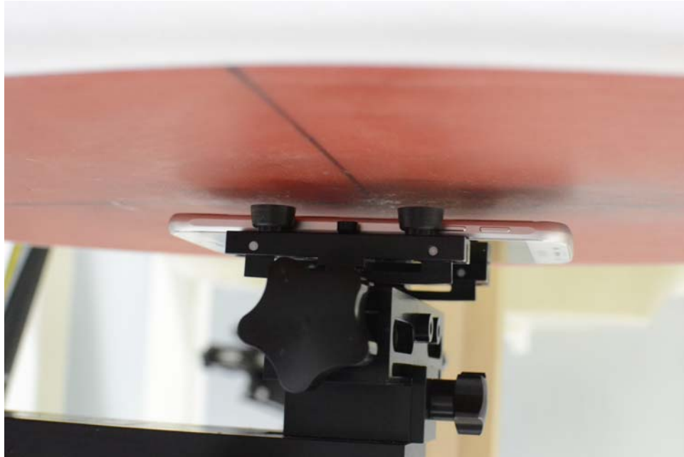
SAR Test Setup Photo 5: Back at 1.0 cm
