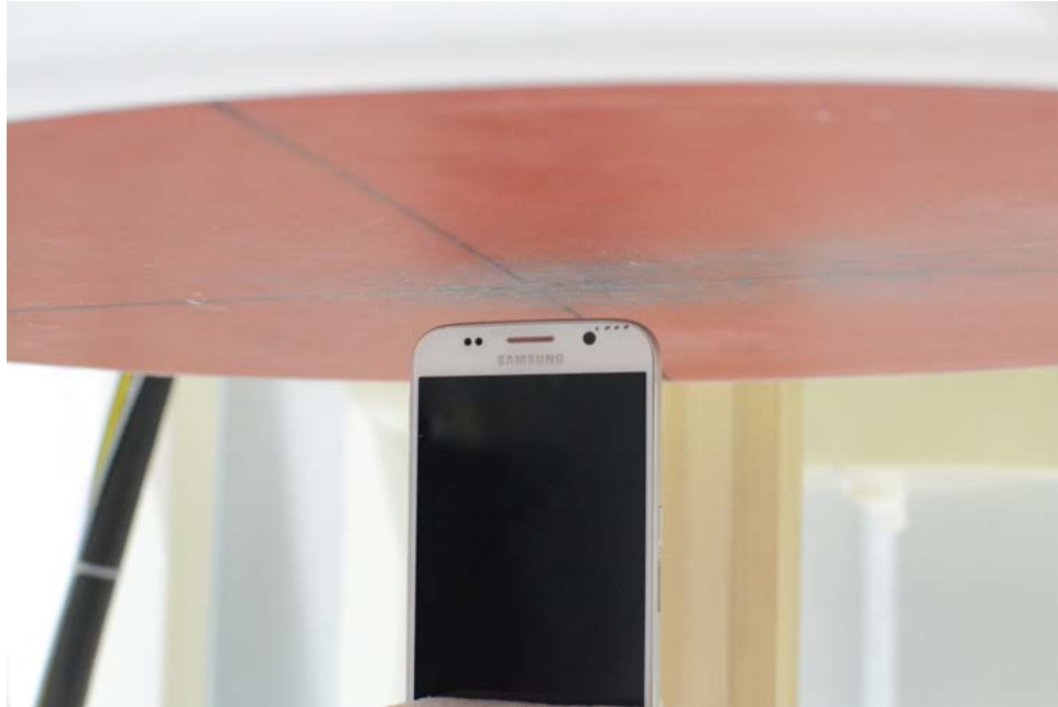
SAR Test Setup Photo 7: Top at 1.0 cm
