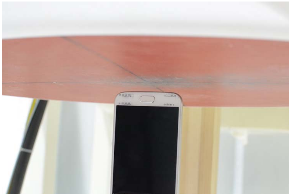
SAR Test Setup Photo 8: Bottom at 1.0 cm
