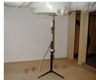
Figure 10-2 System Verification Setup Photo
