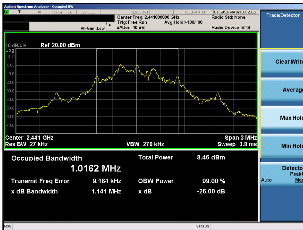
Plot 6-1. Occupied Bandwidth Plot (ANT+ – Ch. 39)
