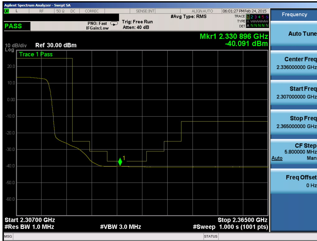
Plot 6-176. Upper Extended Band Edge Plot (Band 30 – 10MHz QPSK – RB Size 50)
