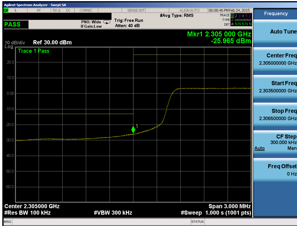
Plot 6-170. Lower Band Edge Plot (Band 30 – 10MHz QPSK – RB Size 50)
