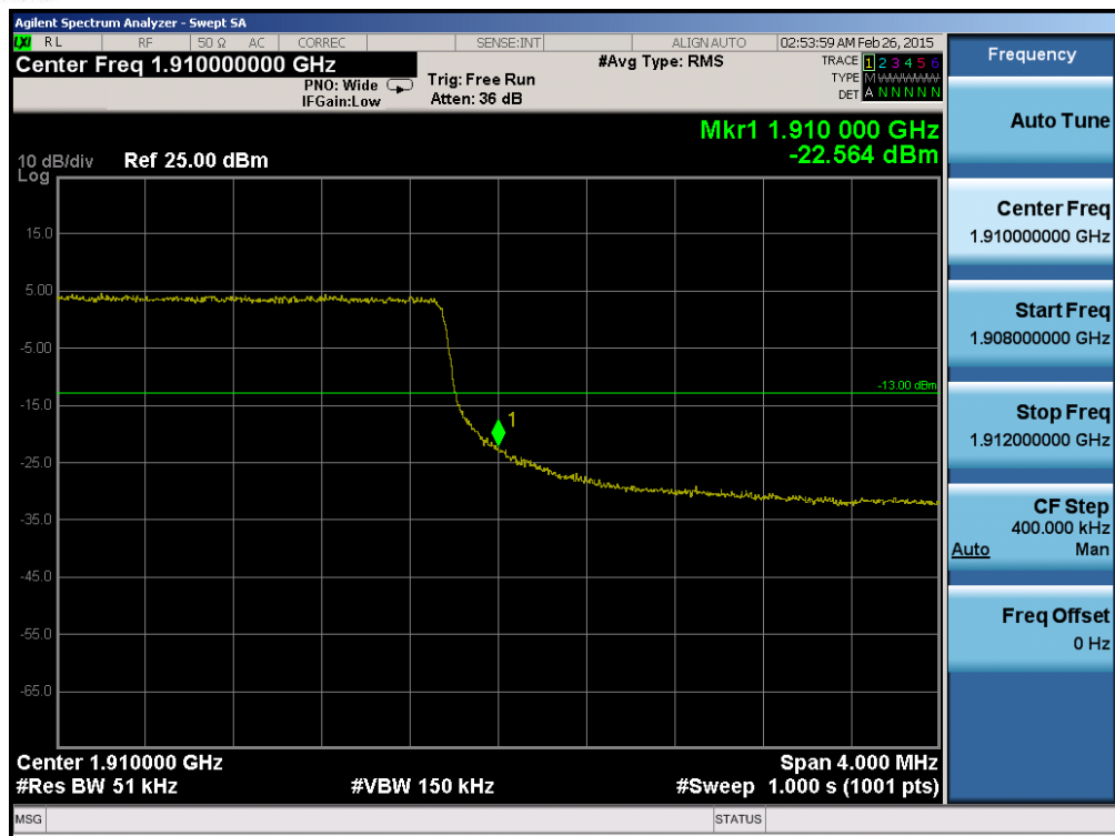
Plot 6-152. Upper Band Edge Plot (Band 2 – 5.0MHz QPSK – RB Size 25)
