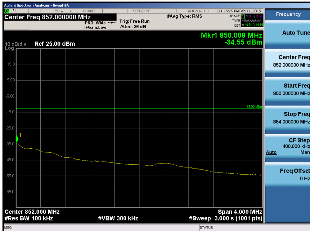
Plot 6-115. Upper Extended Band Edge Plot (Band 5 - 5.0MHz QPSK - RB Size 25)
