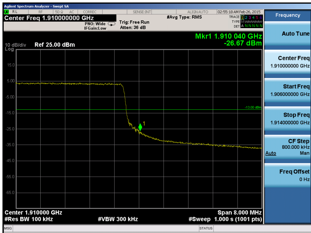
Plot 6-156. Upper Band Edge Plot (Band 2 – 10.0MHz QPSK – RB Size 50)
