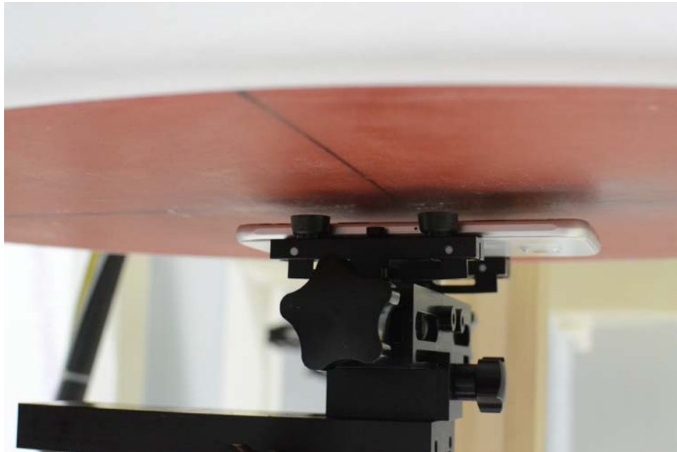
SAR Test Setup Photo 6: Front at 1.0 cm
