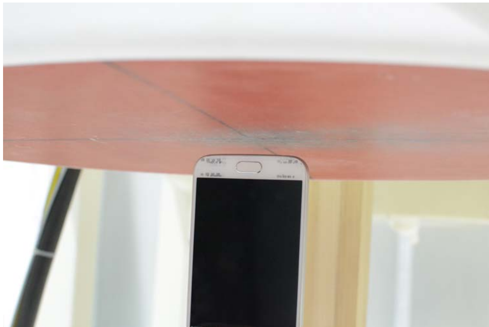
SAR Test Setup Photo 8: Bottom at 1.0 cm
