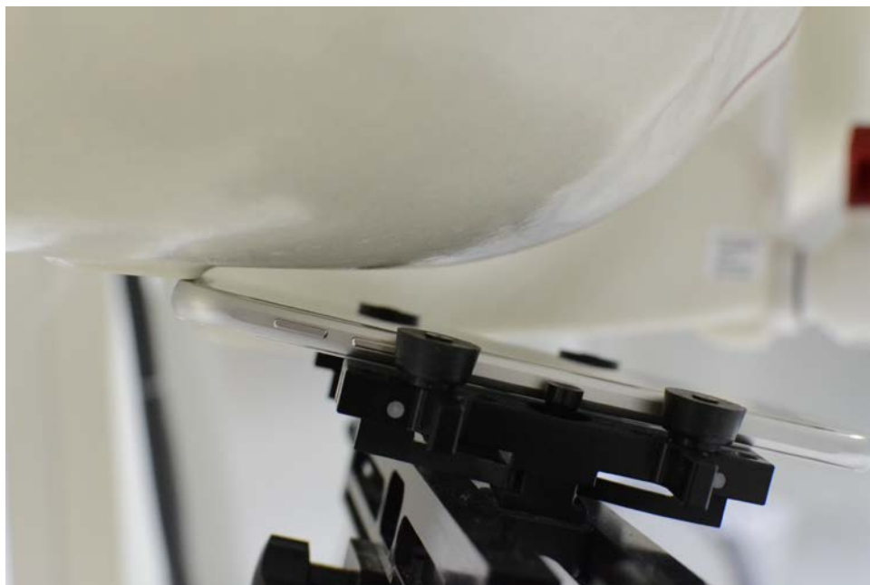
SAR Test Setup Photo 2: Right Tilt
