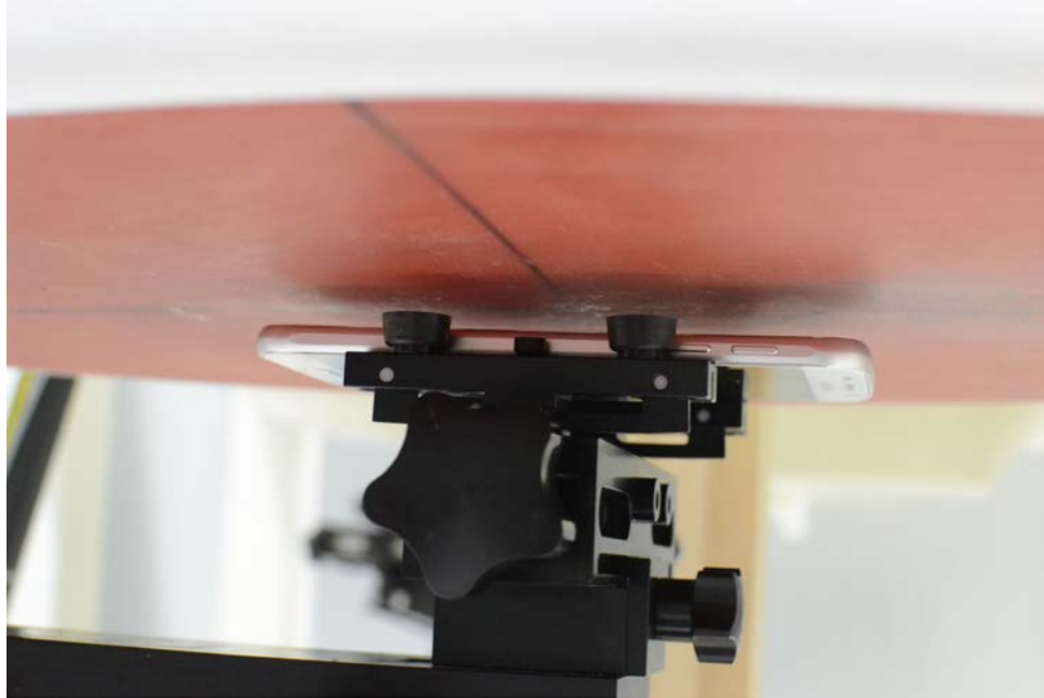
SAR Test Setup Photo 5: Back at 1.0 cm
