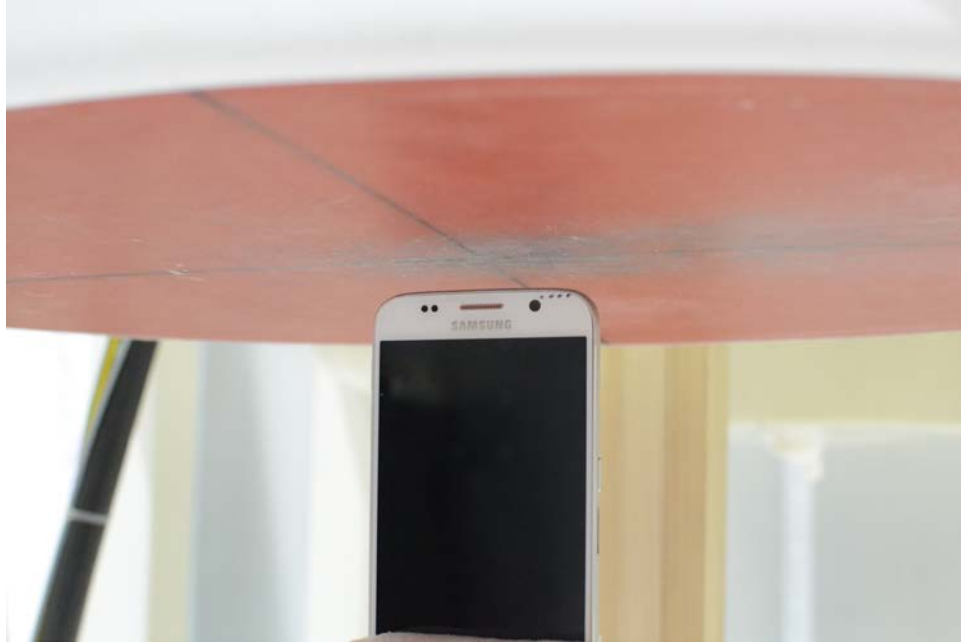
SAR Test Setup Photo 7: Top at 1.0 cm
