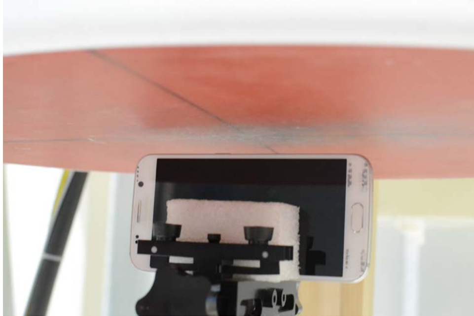
SAR Test Setup Photo 9: Right at 1.0 cm
