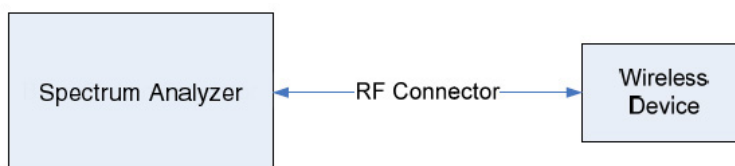
Figure 6-1. Test Instrument & Measurement Setup
