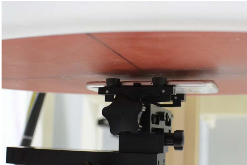
SAR Test Setup Photo 6: Front at 1.0 cm
