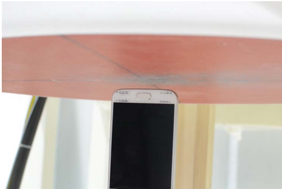
SAR Test Setup Photo 8: Bottom at 1.0 cm
