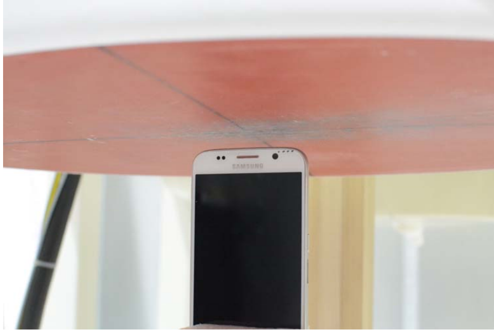
SAR Test Setup Photo 7: Top at 1.0 cm
