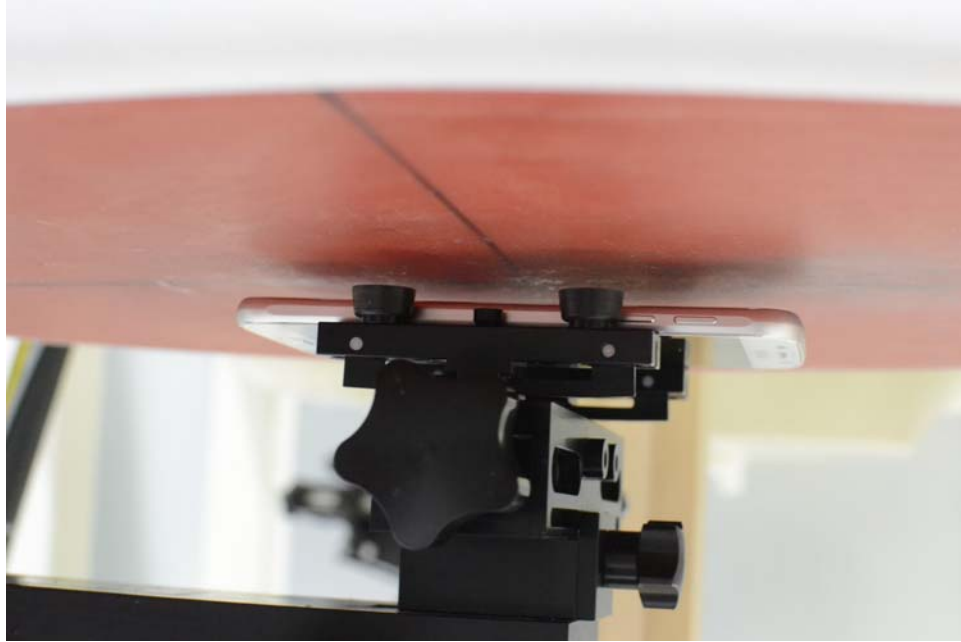
SAR Test Setup Photo 5: Back at 1.0 cm
