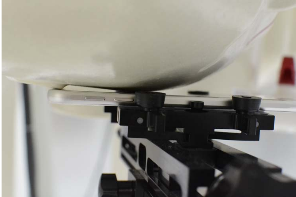
SAR Test Setup Photo 1: Right Cheek
