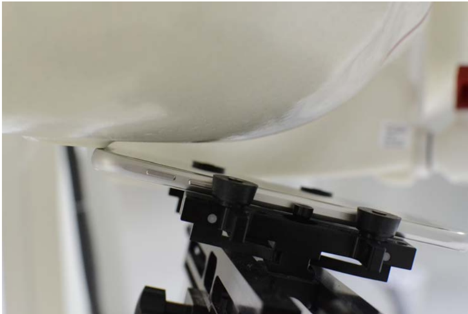
SAR Test Setup Photo 2: Right Tilt
