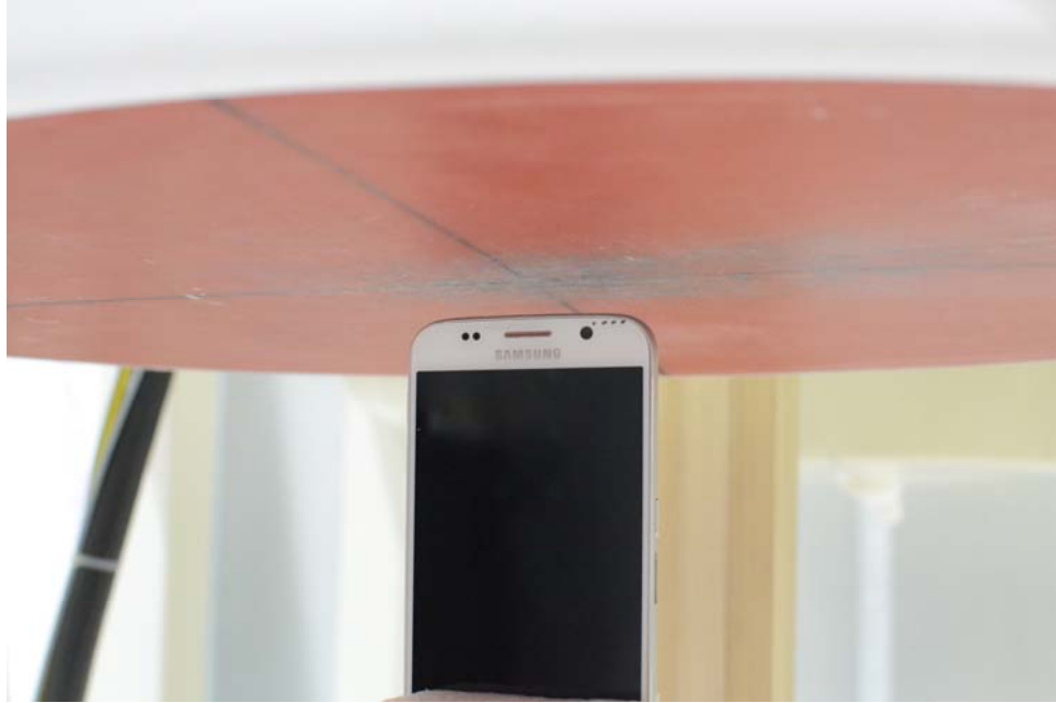
SAR Test Setup Photo 7: Top at 1.0 cm
