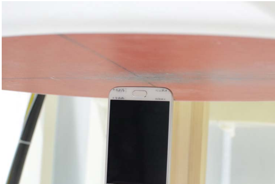
SAR Test Setup Photo 8: Bottom at 1.0 cm
