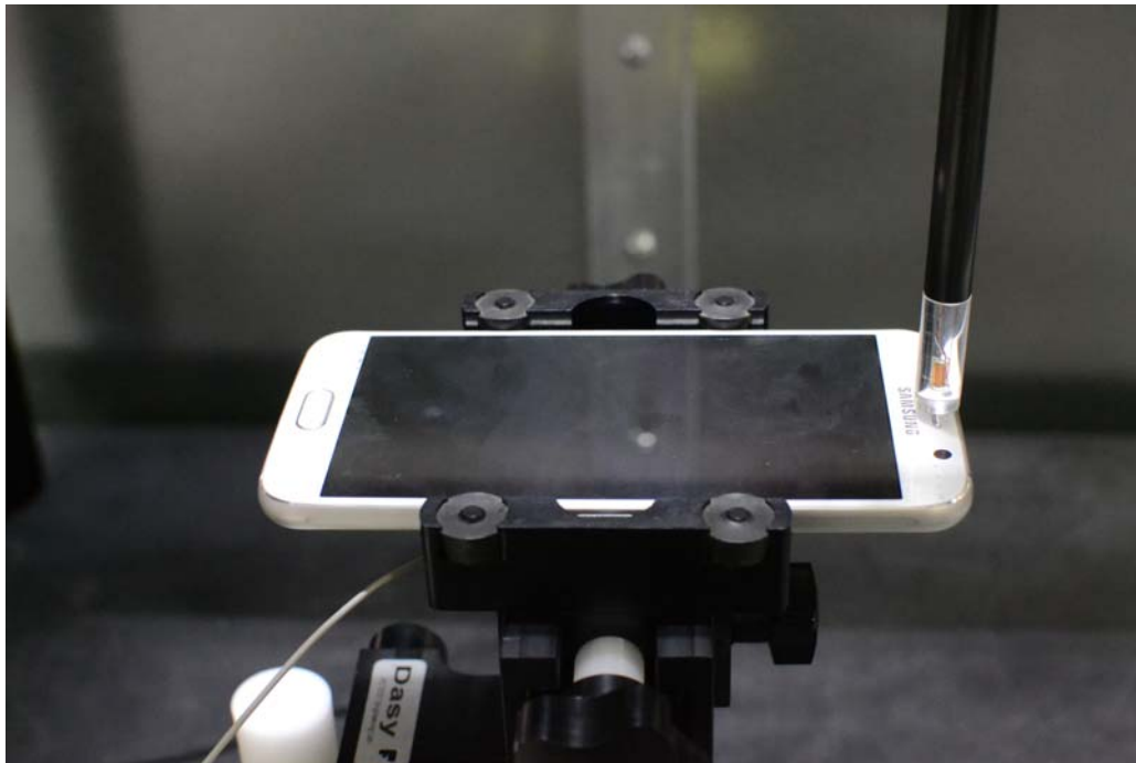
Figure 12-1 Test Setup for Wireless Device
