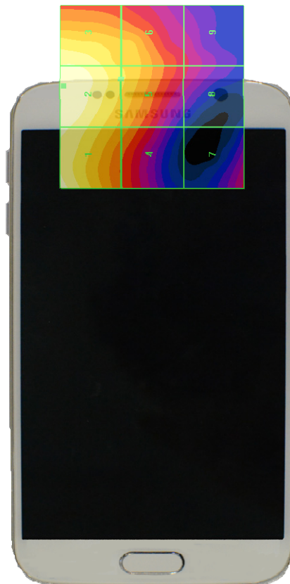
Figure 17-4 E-Field WD Scan overlay
