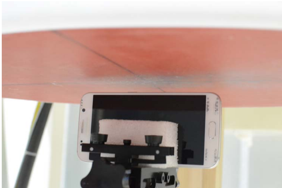
SAR Test Setup Photo 10: Right at 1.0 cm
