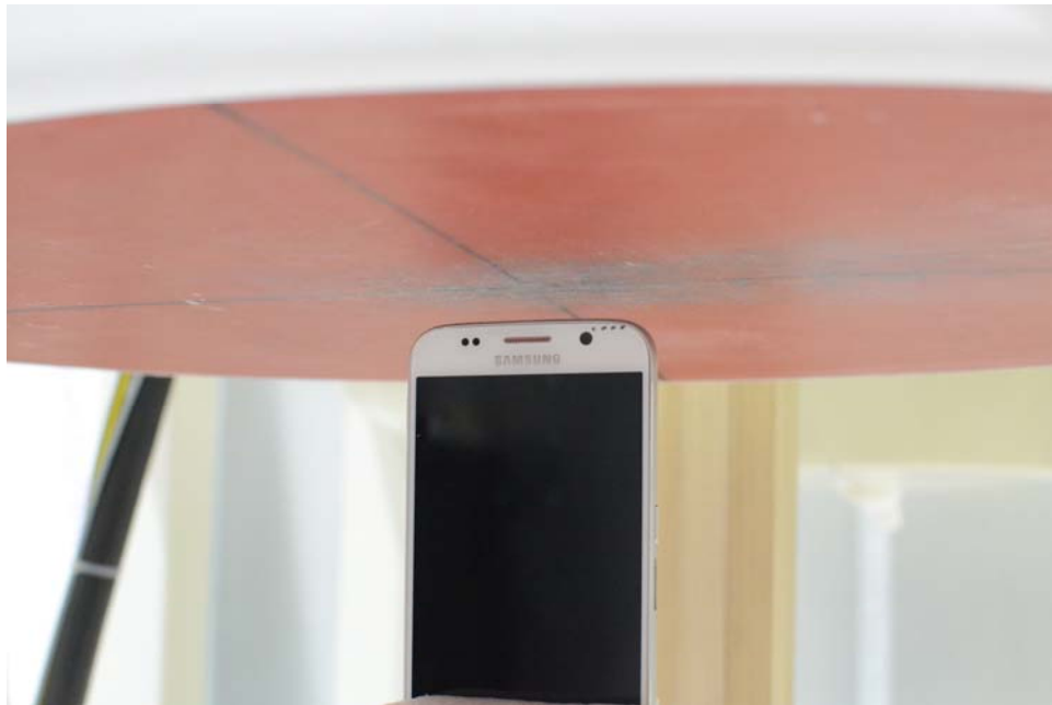
SAR Test Setup Photo 8: Top at 1.0 cm
