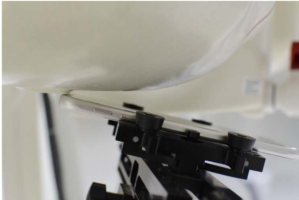
SAR Test Setup Photo 2: Right Tilt
