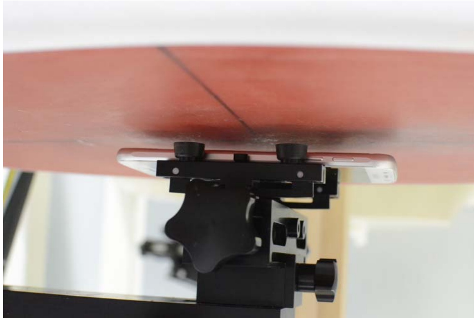
SAR Test Setup Photo 5: Back at 1.0 cm
