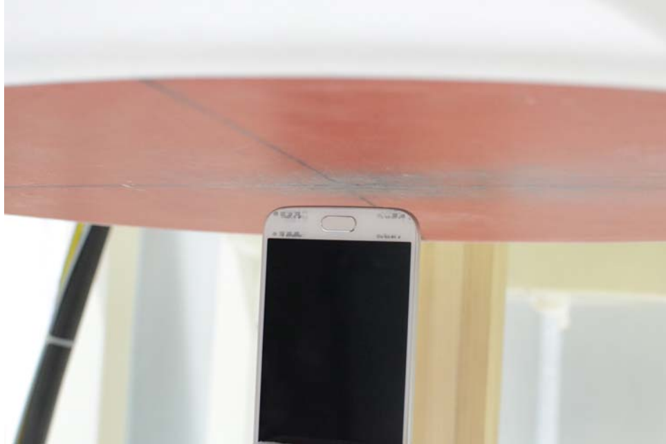
SAR Test Setup Photo 9: Bottom at 1.0 cm
