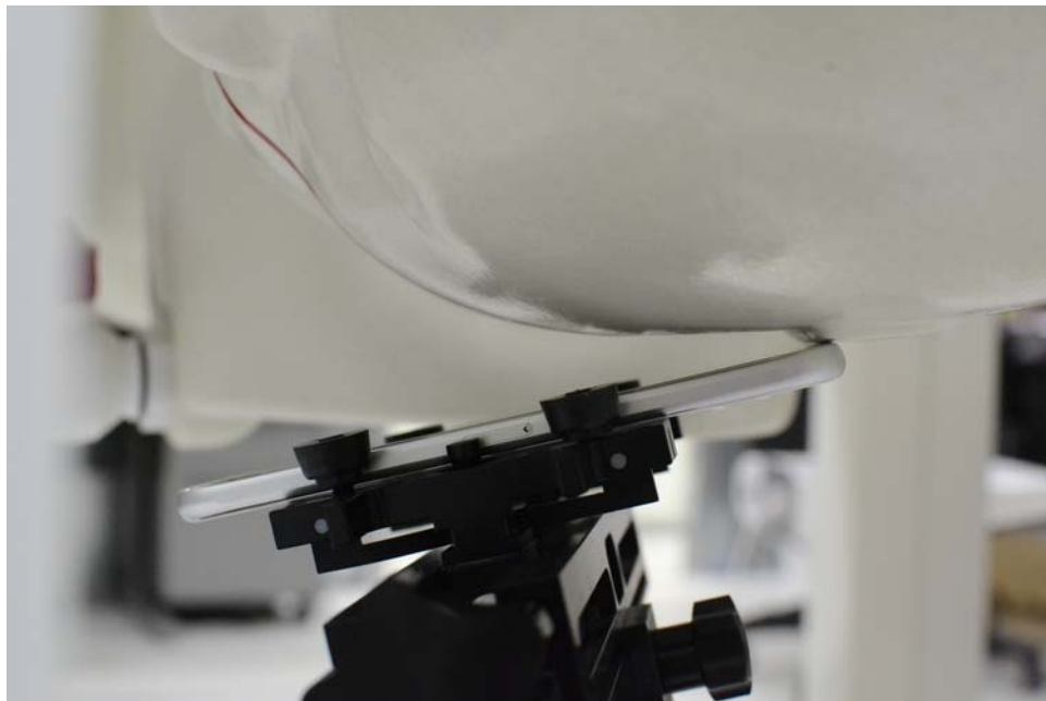
SAR Test Setup Photo 4: Left Tilt
