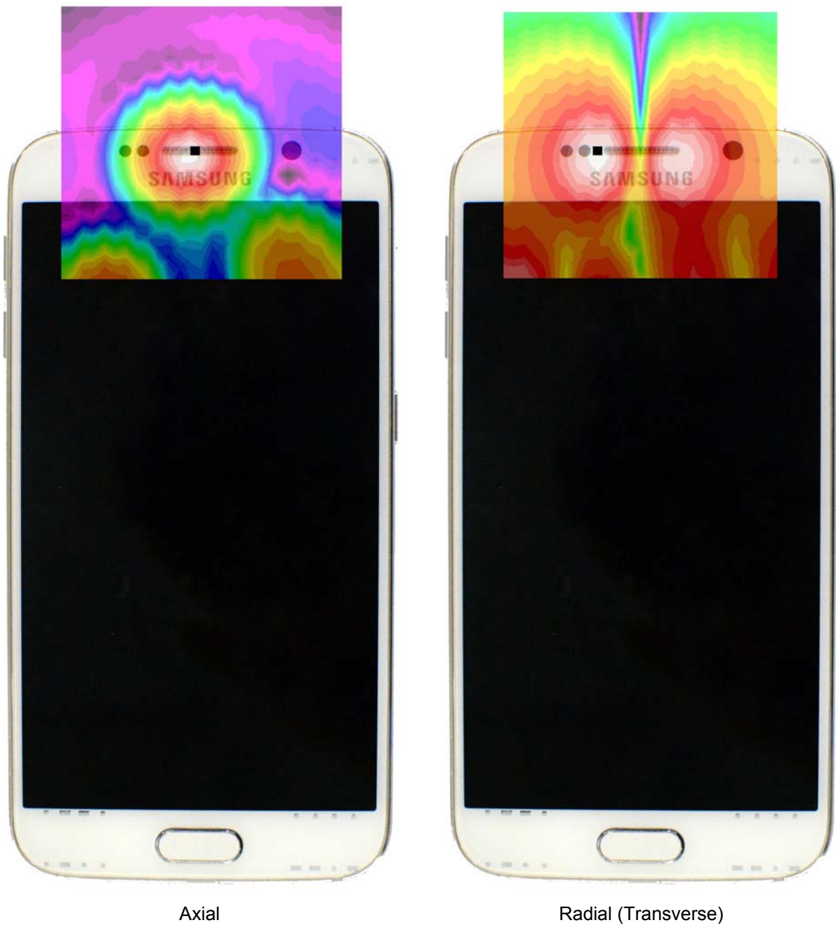
Figure 12-3 T-Coil Scan Overlay Magnetic Field Distributions
