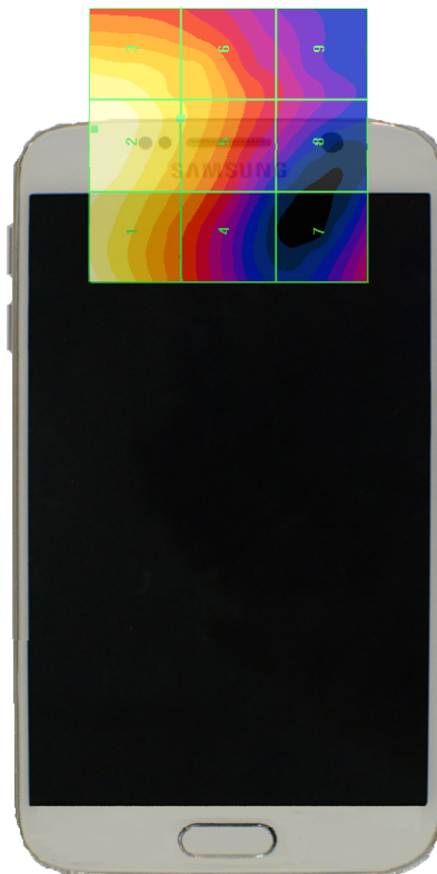
Figure 17-4 E-Field WD Scan overlay
