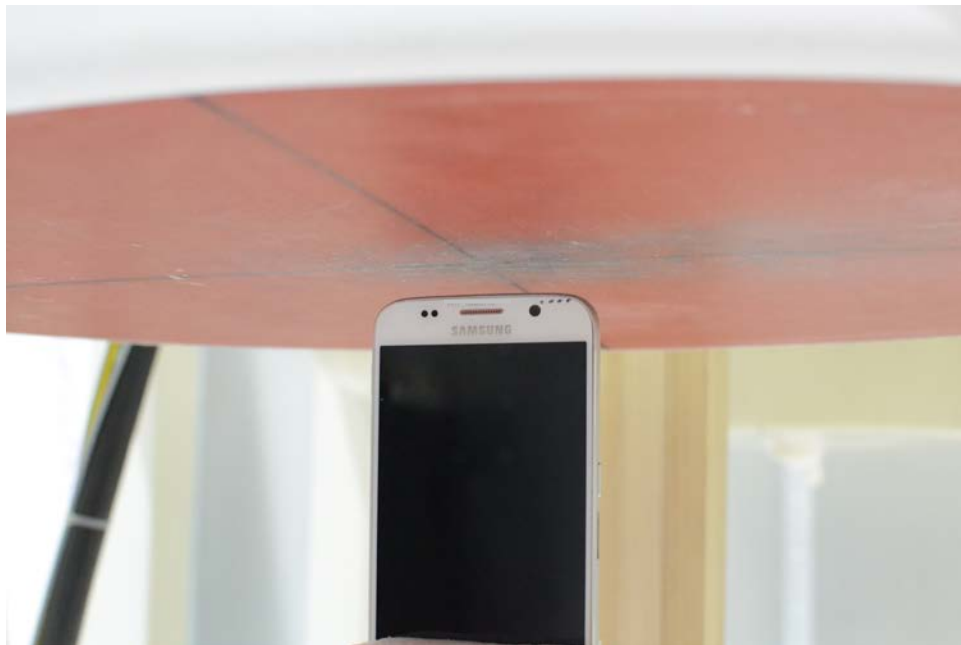
SAR Test Setup Photo 8: Top at 1.0 cm
