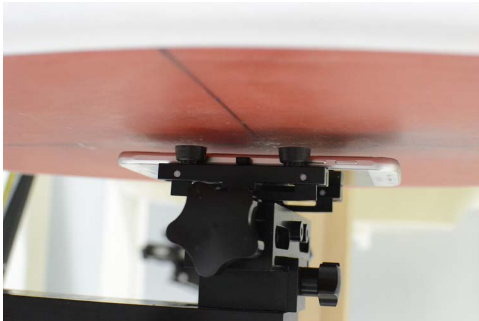
SAR Test Setup Photo 6: Back at 1.0 cm
