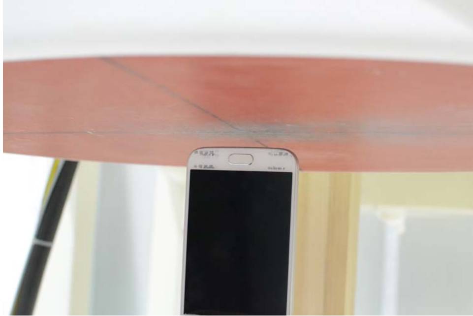
SAR Test Setup Photo 9: Bottom at 1.0 cm
