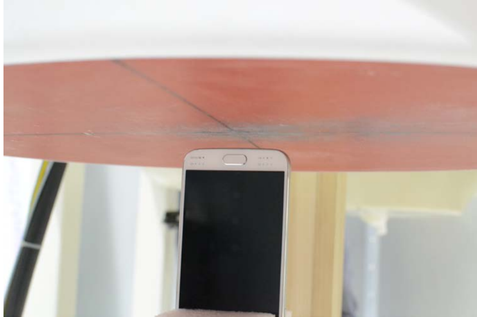
SAR Test Setup Photo 9: Bottom Edge at 10mm
