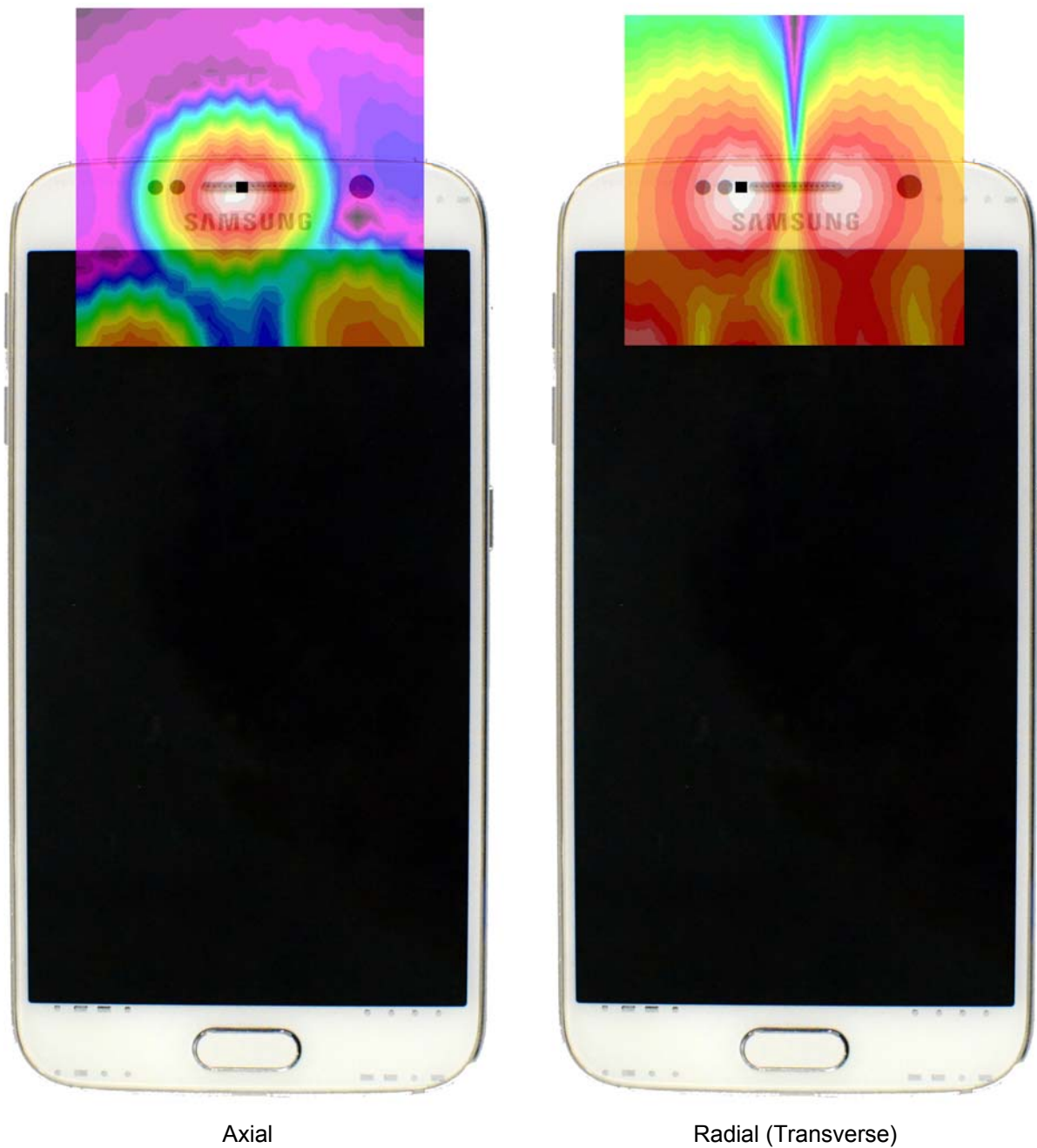
Figure 12-3 T-Coil Scan Overlay Magnetic Field Distributions
