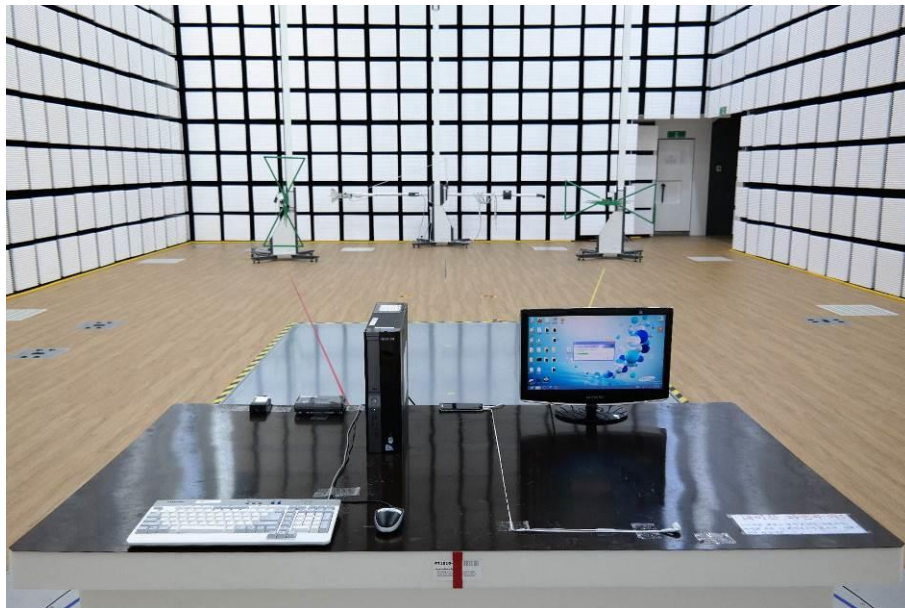
[ Radiated Disturbance for Below 1 GHz – Front ]
