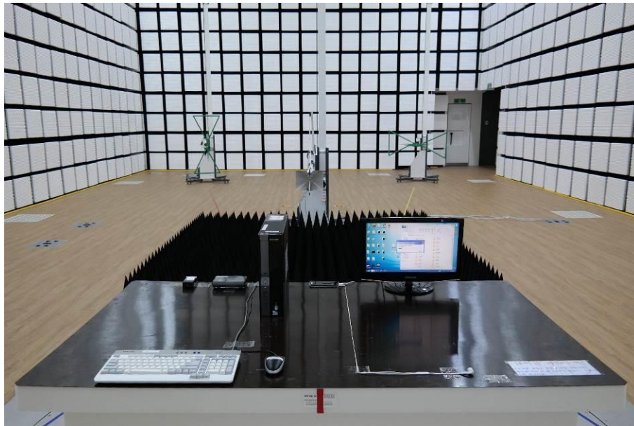
[ Radiated Disturbance for Above 1 GHz – Front ]
