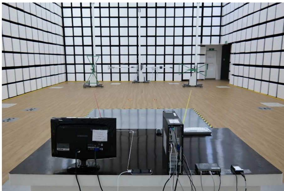
[ Radiated Disturbance for Below 1 GHz – Rear ]
