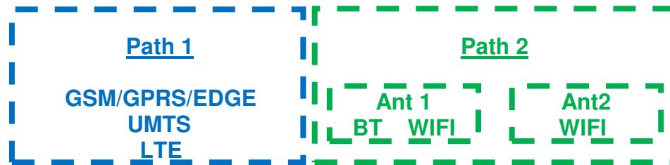
Figure 1-1 Simultaneous Transmission Paths
