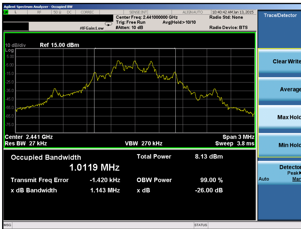
Plot 6-1. Occupied Bandwidth Plot (ANT+ – Ch. 39)
