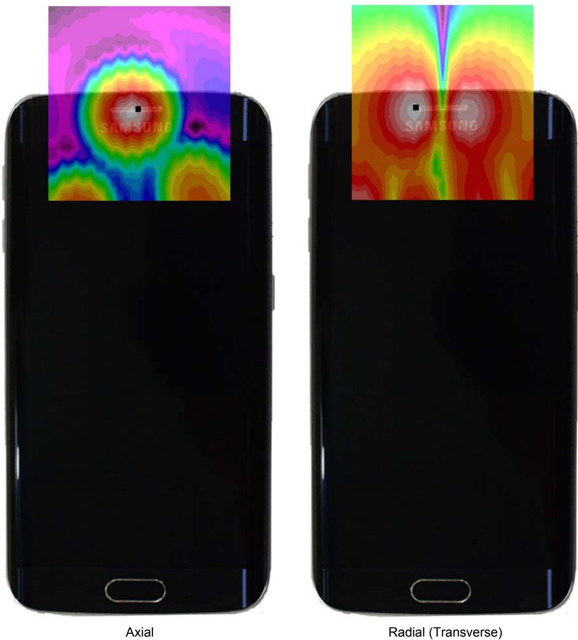
Figure 12-3 T-Coil Scan Overlay Magnetic Field Distributions
