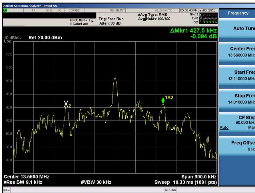
Figure 7-2. 20dB Bandwidth Plot
