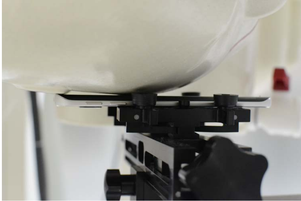
SAR Test Setup Photo 1 – Right Cheek
