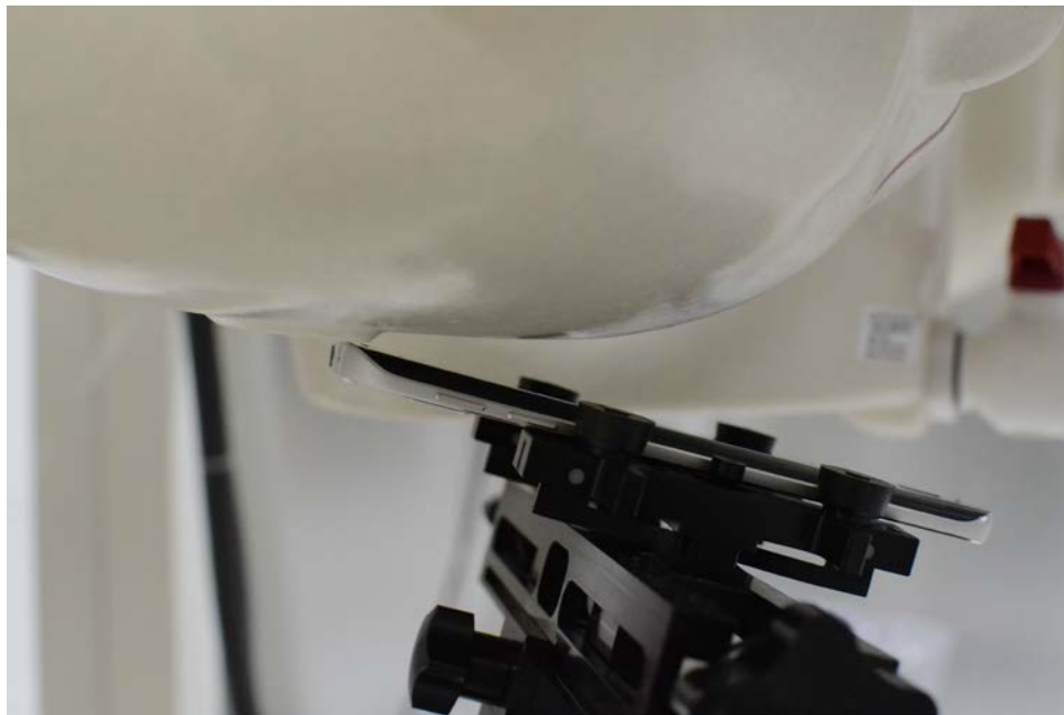
SAR Test Setup Photo 2 – Right Tilt
