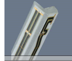
Figure 4-1 E-field Free-space Probe
