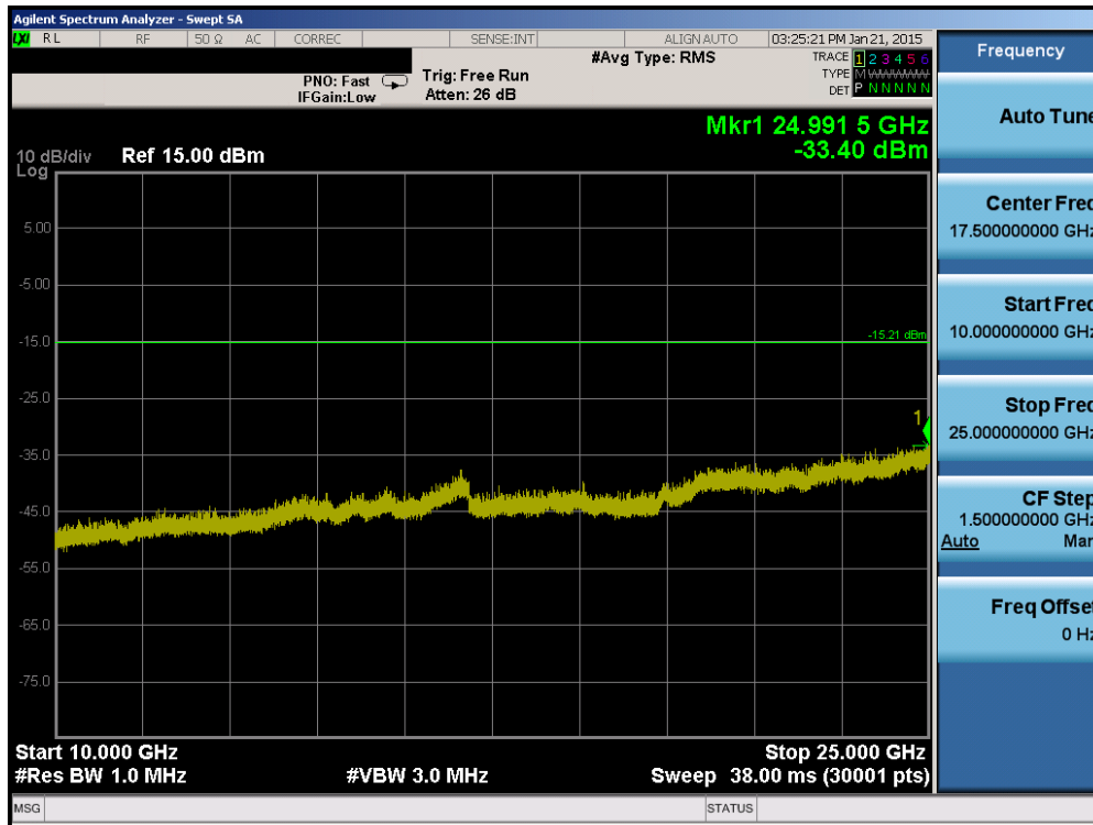
Plot 6-39. Conducted Spurious Plot (Bluetooth, 1Mbps – Ch. 39)
