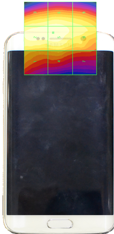
Figure 17-4 E-Field WD Scan overlay
