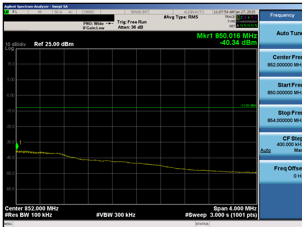
Plot 6-111. Upper Extended Band Edge Plot (Band 5 – 1.4MHz QPSK – RB Size 6)
