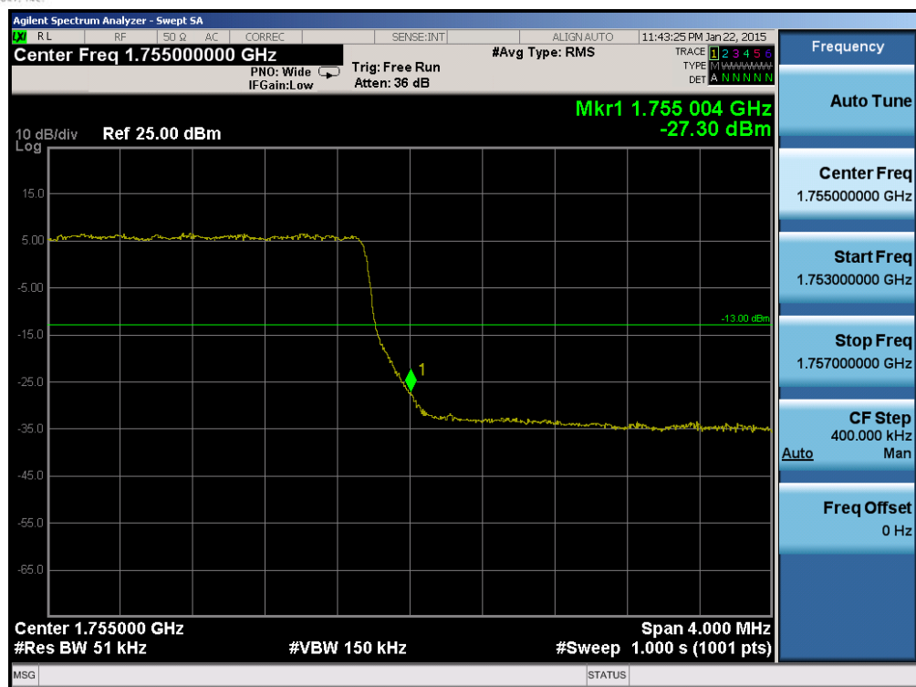
Plot 6-132. Upper Band Edge Plot (Band 4 – 5.0MHz QPSK – RB Size 25)
