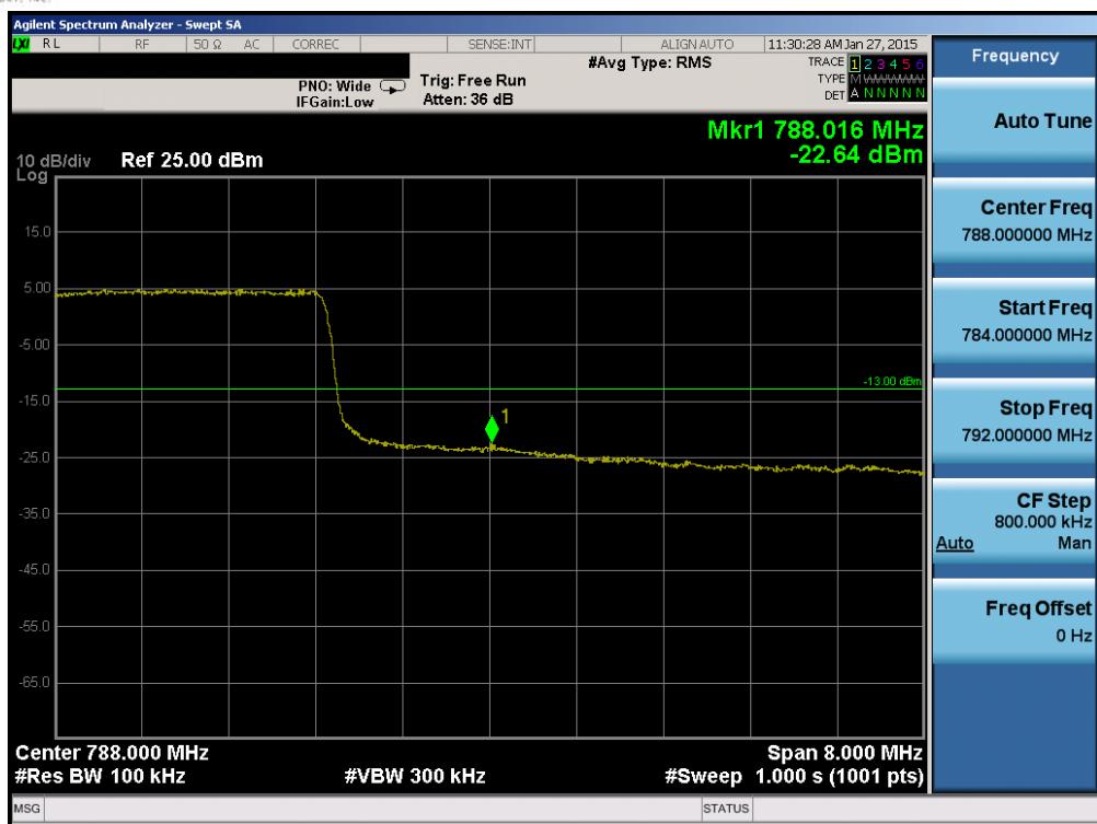
Plot 6-106. Upper Band Edge Plot (Band 13 – 10.0MHz QPSK – RB Size 50)
