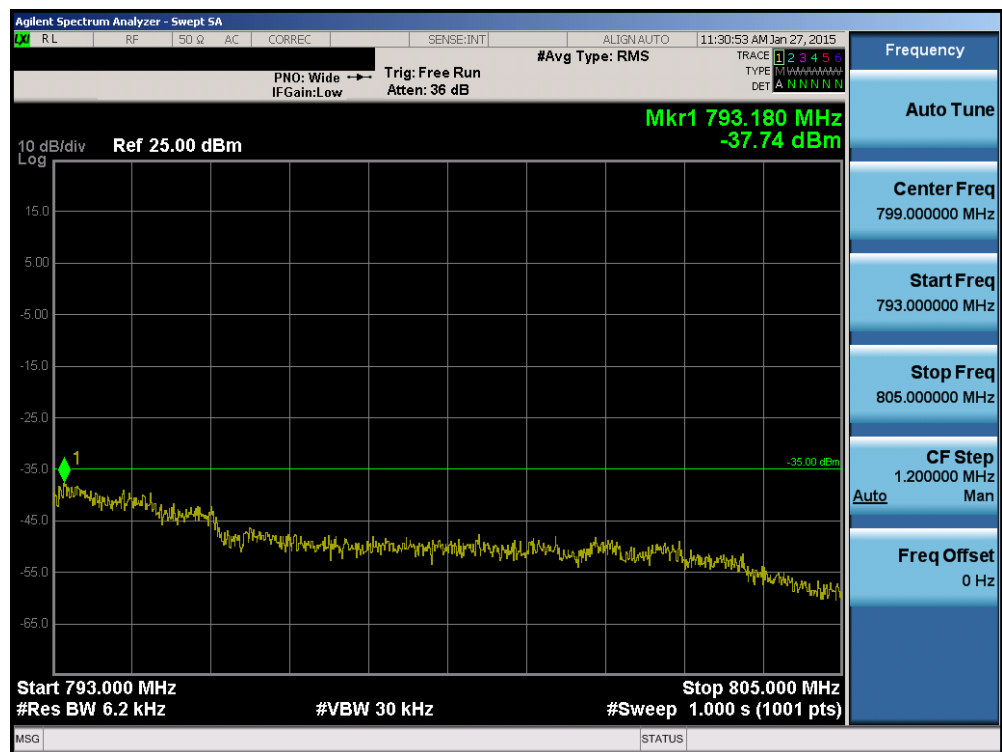
Plot 6-107. Upper Emission Mask Plot (Band 13 – 10.0MHz QPSK – RB Size 50)
