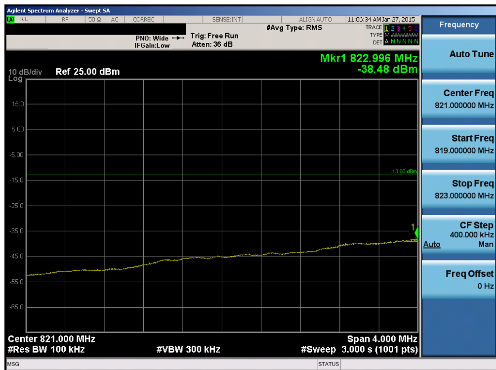
Plot 6-109. Lower Extended Band Edge Plot (Band 5 – 1.4MHz QPSK – RB Size 6)
