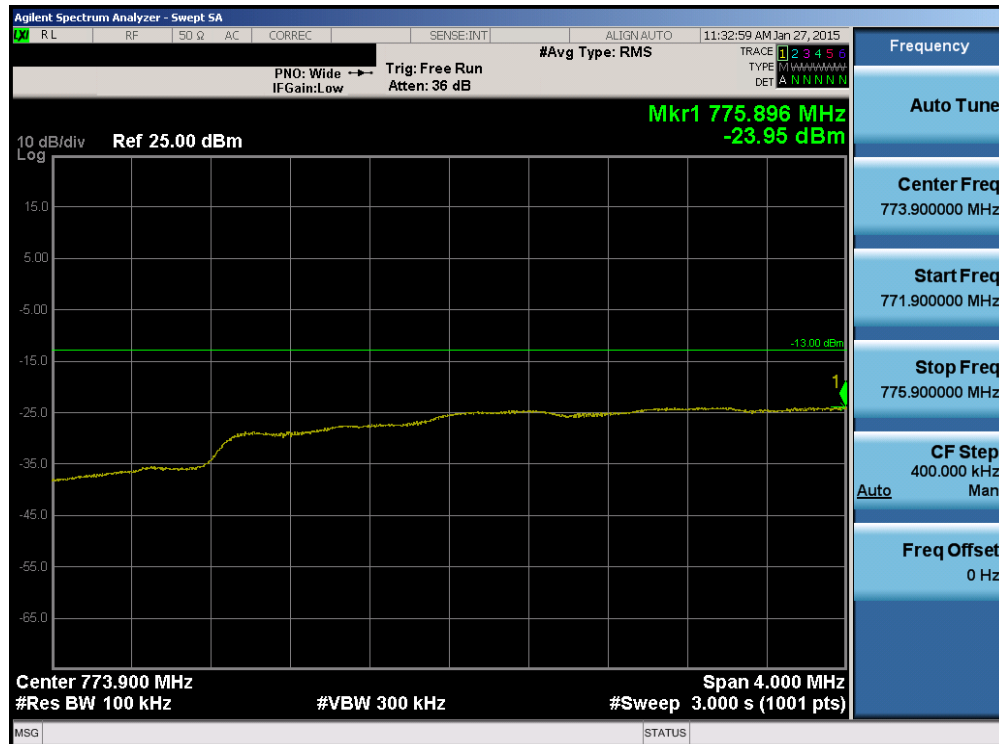
Plot 6-99. Lower Extended Band Edge Plot (Band 13 – 5.0MHz QPSK – RB Size 25)
