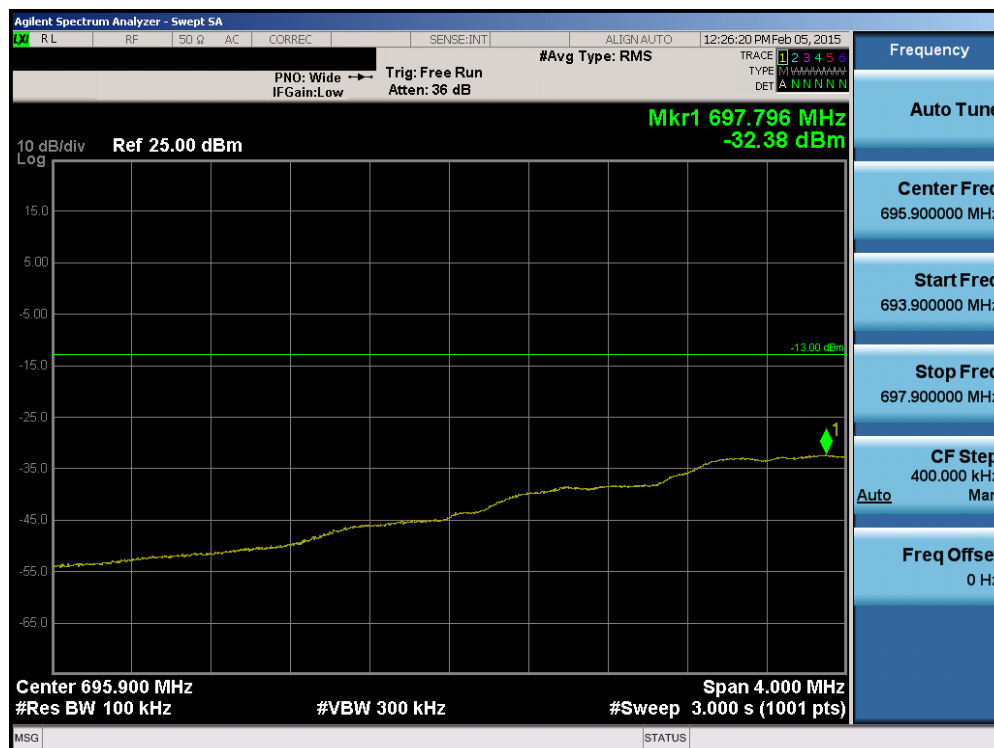
Plot 6-85. Lower Extended Band Edge Plot (Band 12 – 1.4MHz QPSK – RB Size 6)
