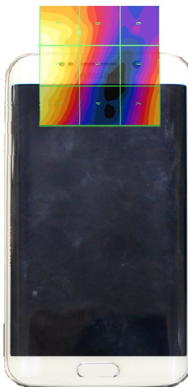
Figure 17-4 E-Field WD Scan overlay
