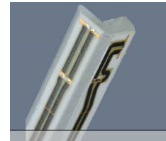
Figure 4-1 E-field Free-space Probe
