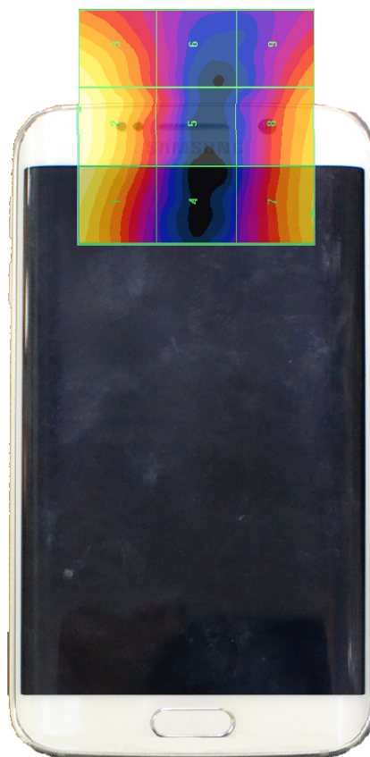
Figure 17-4 E-Field WD Scan overlay
