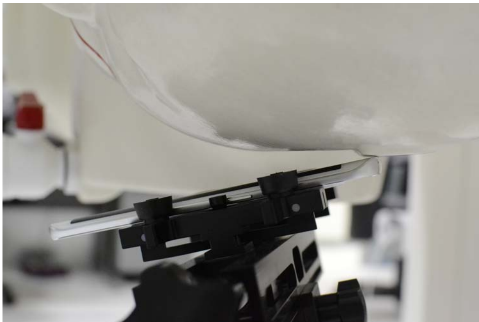
SAR Test Setup Photo 4: Left Tilt
