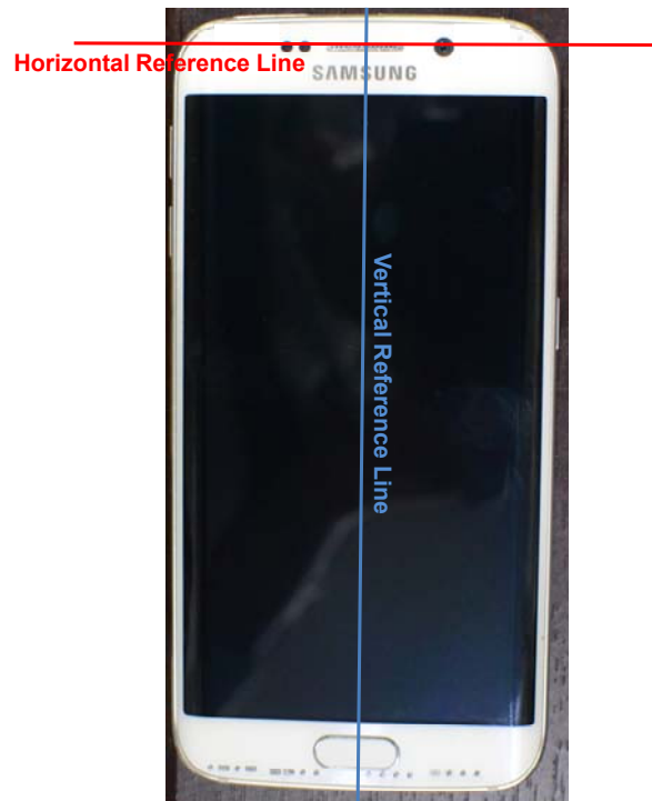
SAR Test Setup Photo 12: Horizontal and Vertical Reference Lines
