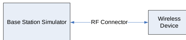
Figure 9-2 Power Measurement Setup
