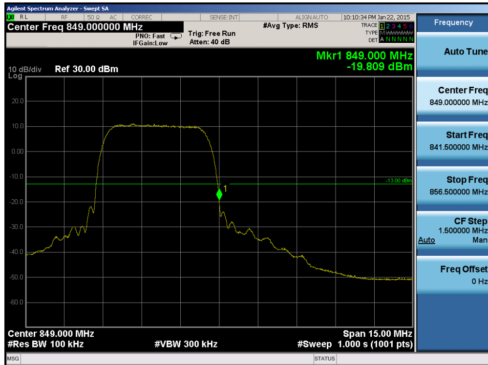
Plot 6-78. Band Edge Plot (Cellular WCDMA Mode – Ch. 4233)
