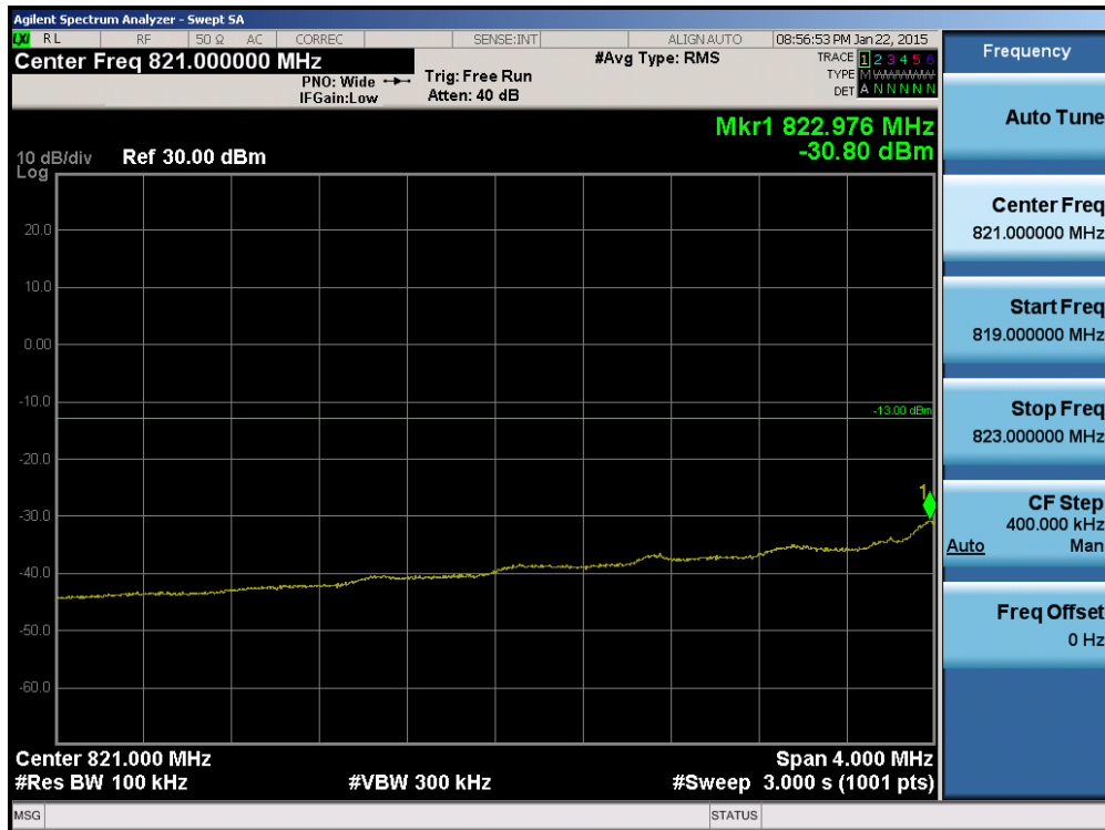
Plot 6-70. 4MHz Span Plot (Cellular CDMA Mode – Ch. 1013)
