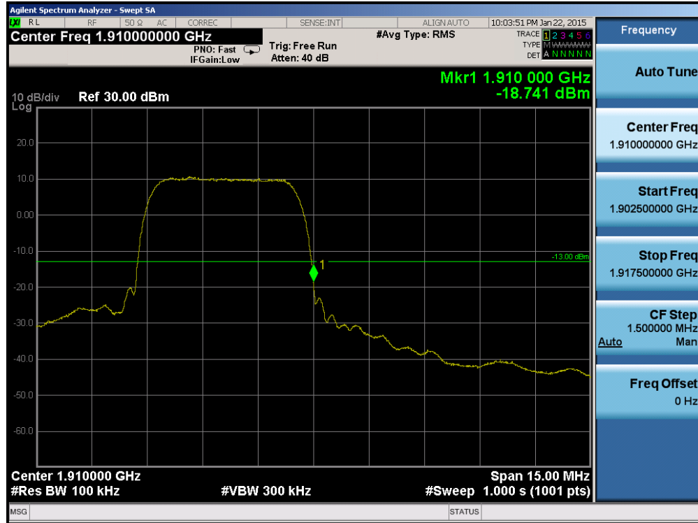
Plot 6-81. Band Edge Plot (PCS WCDMA Mode – Ch. 9538)
