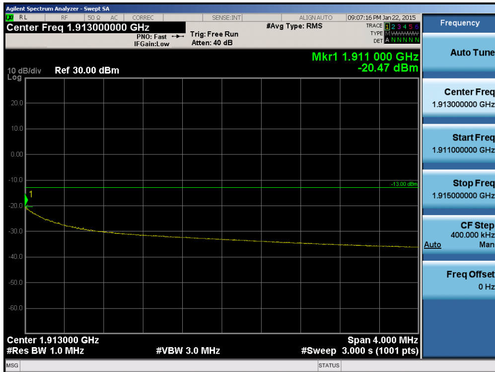
Plot 6-76. 4MHz Span Plot (PCS CDMA Mode – Ch. 1175)
