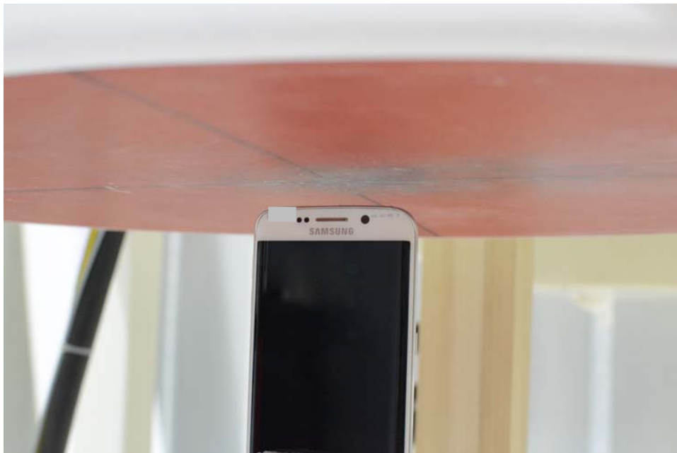
SAR Test Setup Photo 8: Top Edge at 10mm
