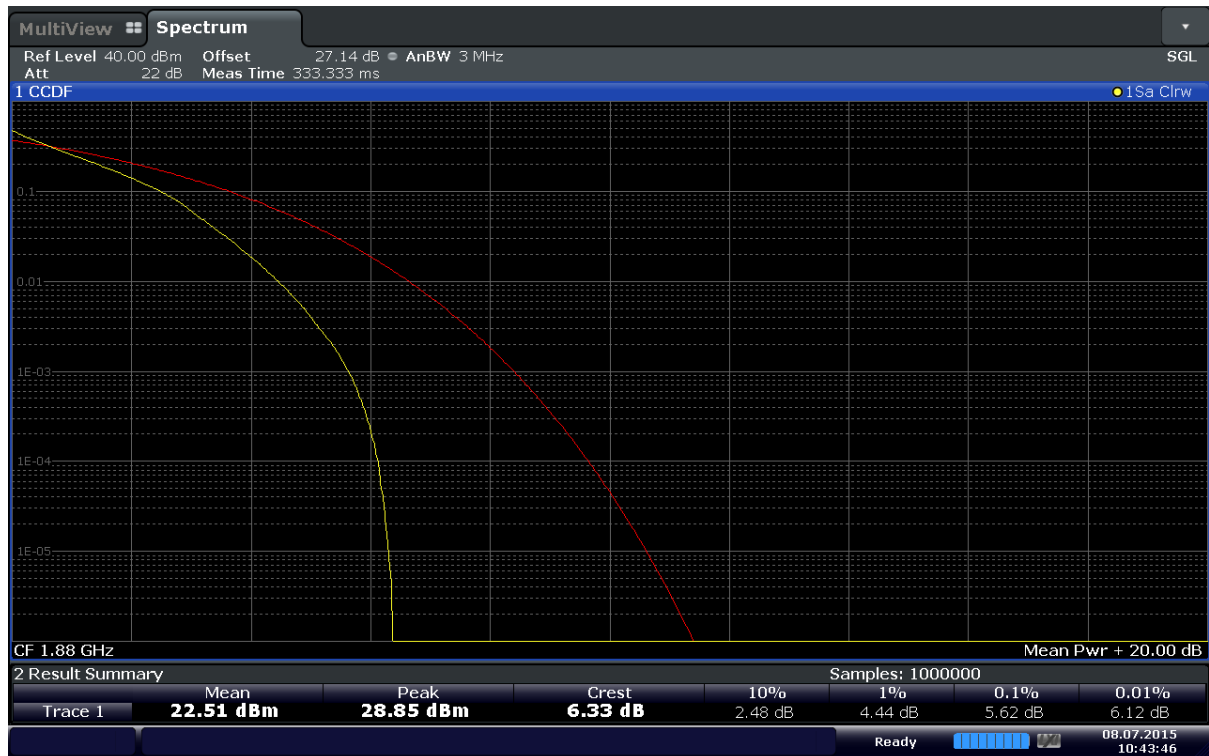
Plot 6-152. Peak-Average Ratio Plot (Band 2 – 3.0MHz QPSK - RB Size 15)
