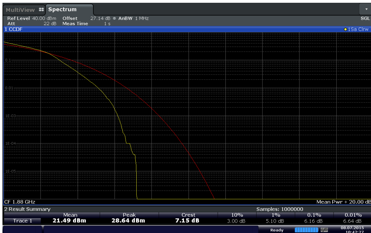
Plot 6-151. Peak-Average Ratio Plot (Band 2 – 1.4MHz 16QAM - RB Size 6)
