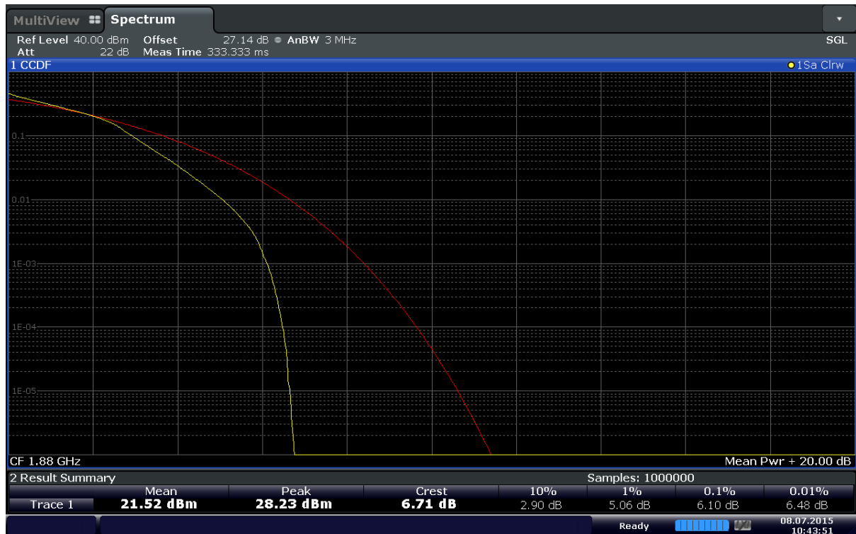
Plot 6-153. Peak-Average Ratio Plot (Band 2 – 3.0MHz 16QAM - RB Size 15)
