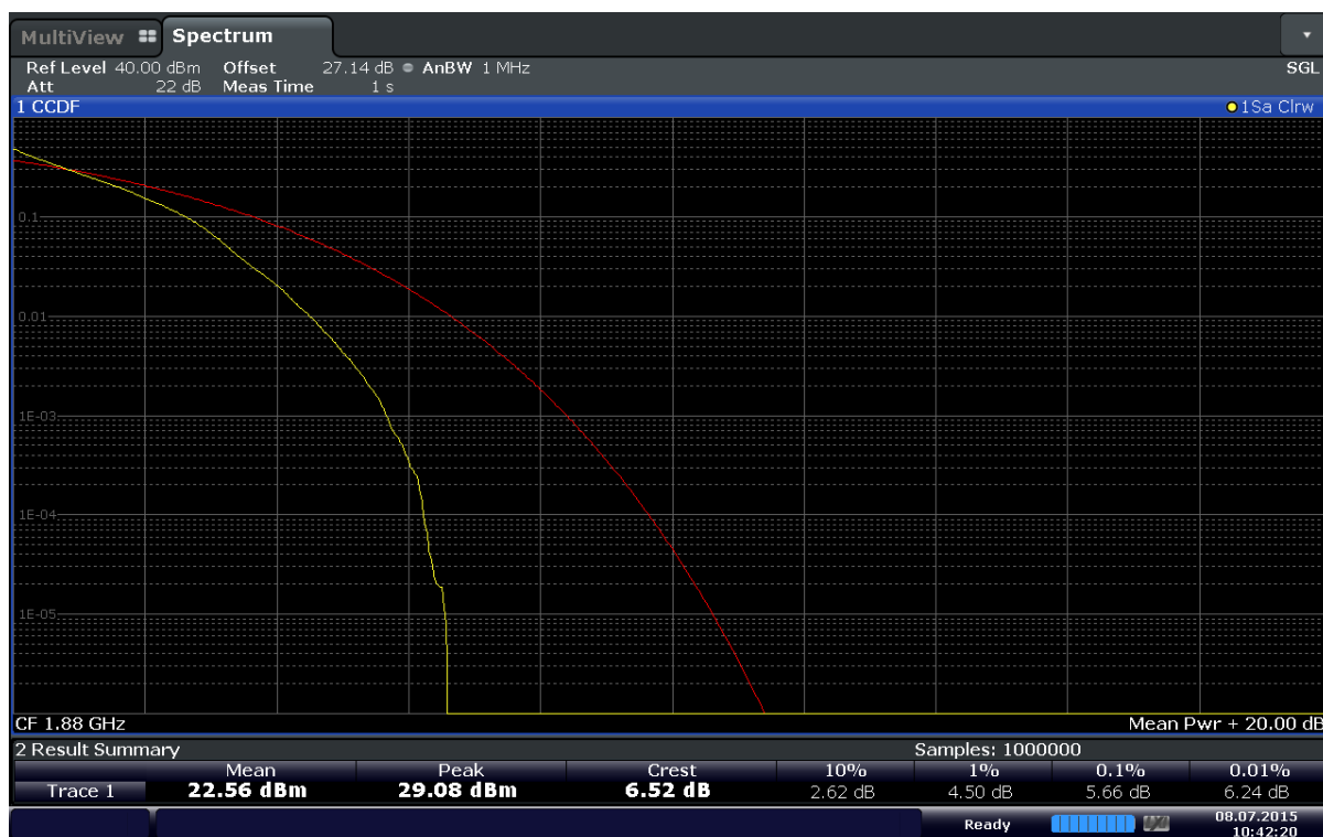
Plot 6-150. Peak-Average Ratio Plot (Band 2 – 1.4MHz QPSK - RB Size 6)
