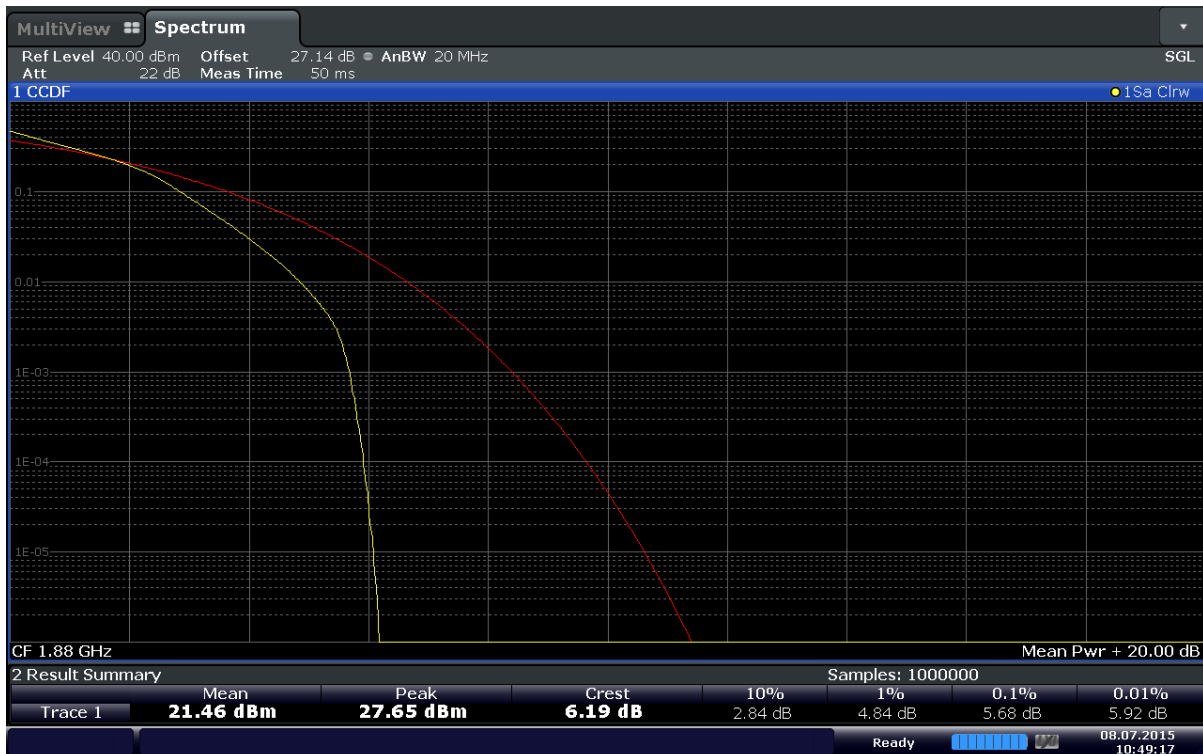
Plot 6-161. Peak-Average Ratio Plot (Band 2 – 20.0MHz 16QAM - RB Size 100)
