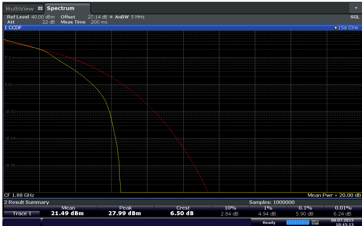
Plot 6-155. Peak-Average Ratio Plot (Band 2 – 5.0MHz 16QAM - RB Size 25)
