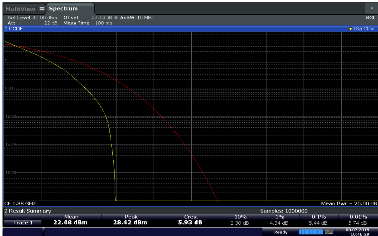
Plot 6-156. Peak-Average Ratio Plot (Band 2 – 10.0MHz QPSK - RB Size 50)
