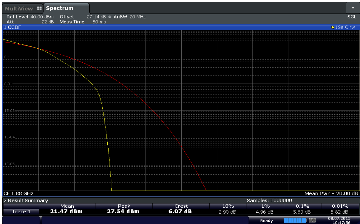
Plot 6-159. Peak-Average Ratio Plot (Band 2 – 15.0MHz 16QAM - RB Size 75)
