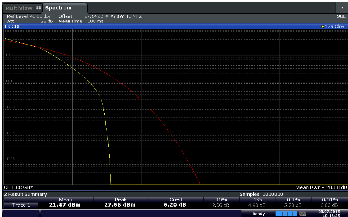
Plot 6-157. Peak-Average Ratio Plot (Band 2 – 10.0MHz 16QAM - RB Size 50)
