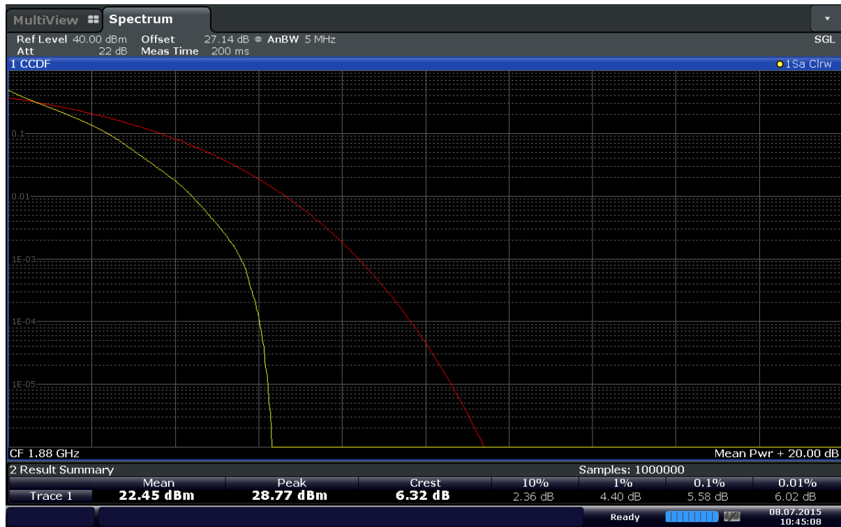
Plot 6-154. Peak-Average Ratio Plot (Band 2 – 5.0MHz QPSK - RB Size 25)
