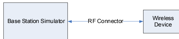
Figure 9-1 Power Measurement Setup
