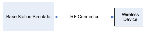
Figure 9-2 Power Measurement Setup
