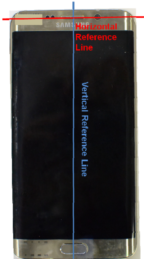
SAR Test Setup Photo 17 – DUT Reference Lines
