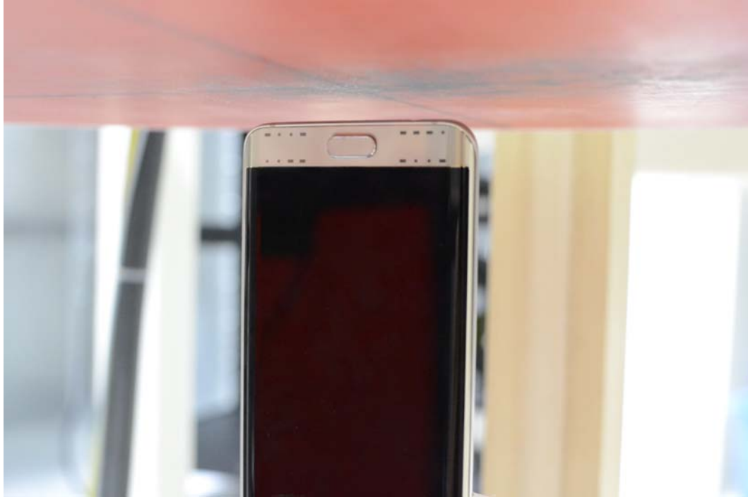
SAR Test Setup Photo 13 – Bottom Edge at 1.0 cm (Hotspot)
