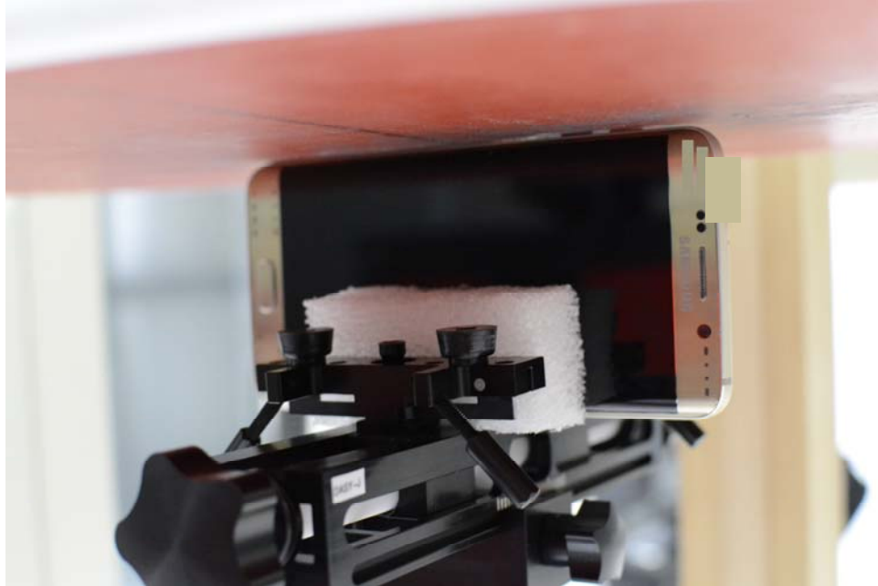
SAR Test Setup Photo 15 – Left Edge at 0.0 cm (Extremity)
