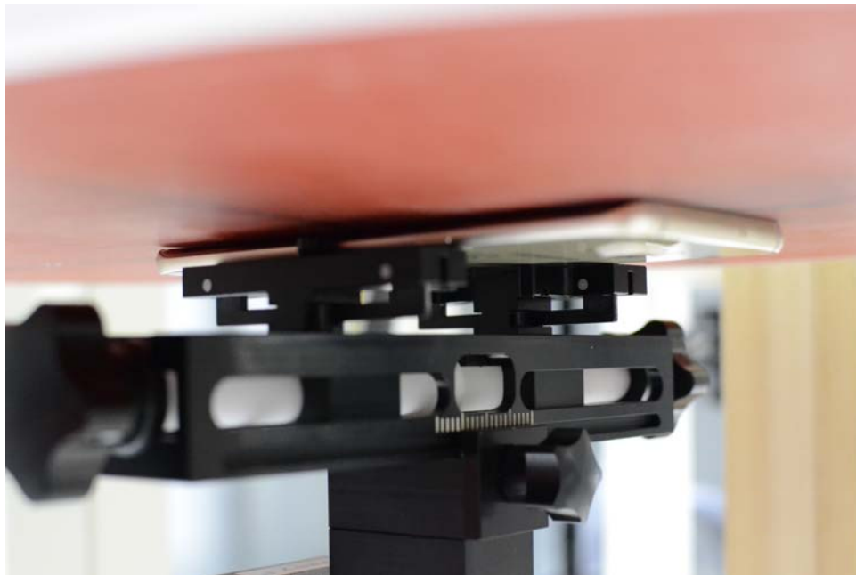
SAR Test Setup Photo 8— Front Side at 0.0 cm (Extremity)
