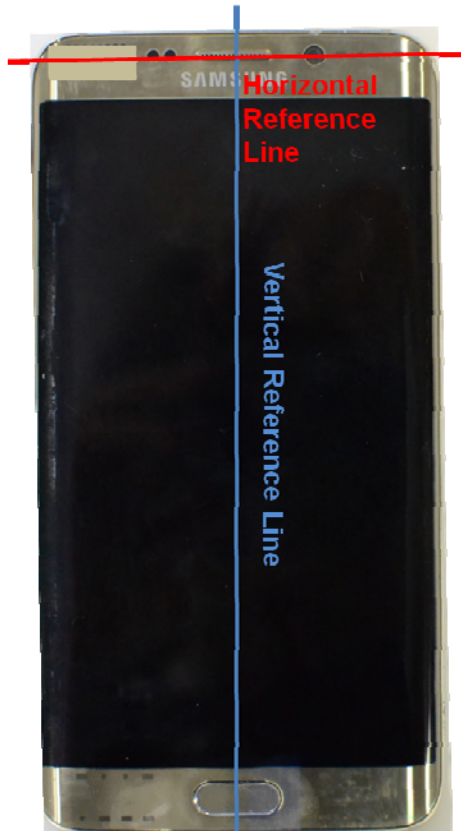
SAR Test Setup Photo 17 – DUT Reference Lines
