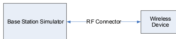
Figure 9-2 Power Measurement Setup
