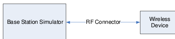
Figure 9-2 Power Measurement Setup
