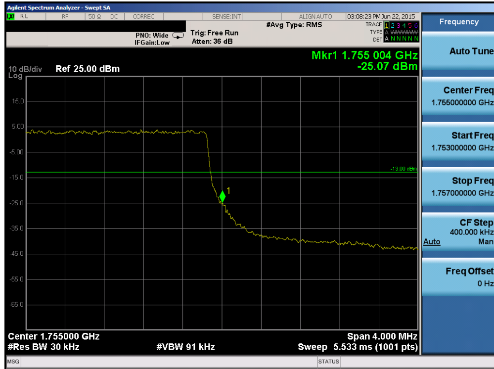
Plot 6-115. Upper Band Edge Plot (Band 4 – 3.0MHz QPSK – RB Size 15)
