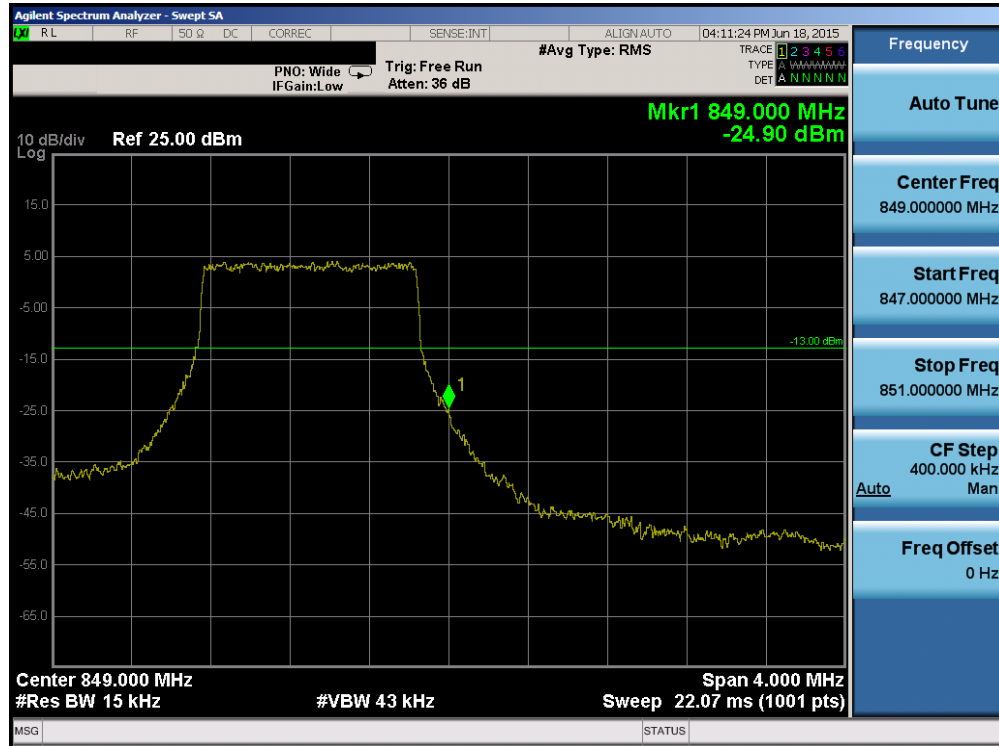
Plot 6-95. Upper Band Edge Plot (Band 5/26 – 1.4MHz QPSK – RB Size 6)
