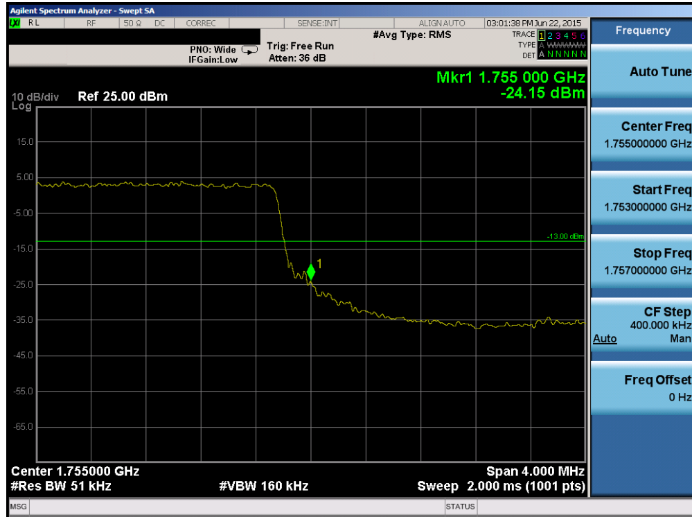
Plot 6-119. Upper Band Edge Plot (Band 4 – 5.0MHz QPSK – RB Size 25)
