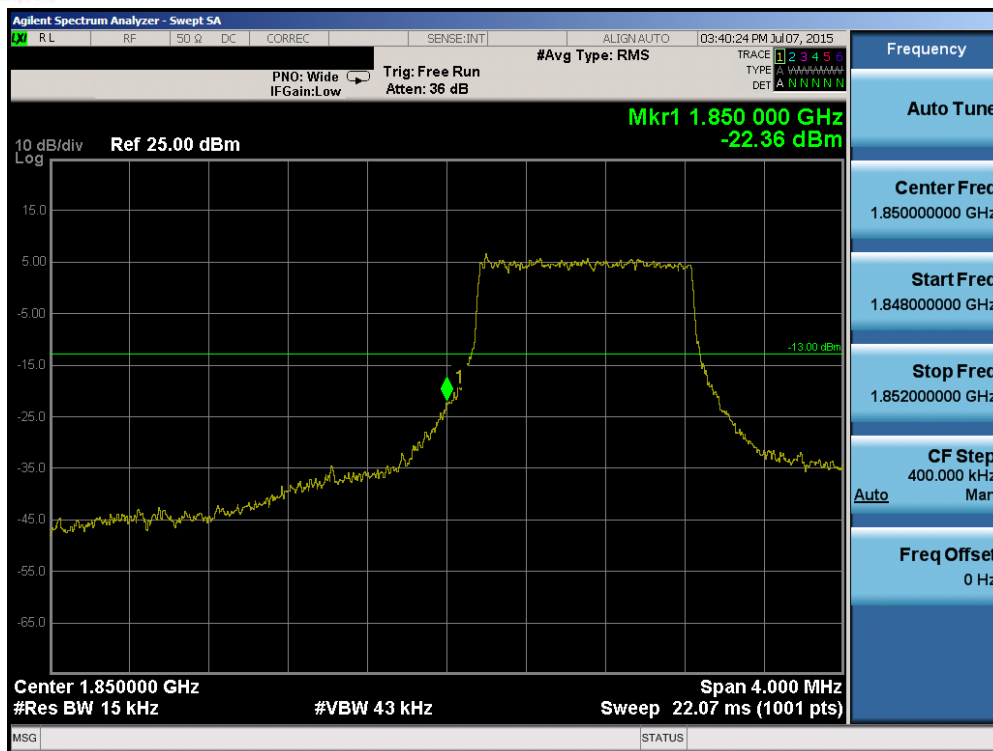
Plot 6-133. Lower Band Edge Plot (Band 2 – 1.4MHz QPSK – RB Size 6)
