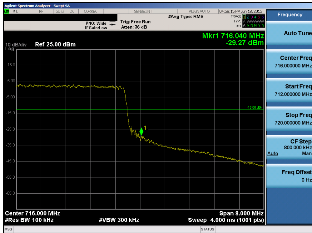
Plot 6-92. Upper Band Edge Plot (Band 12/17 – 10.0MHz QPSK – RB Size 50)
