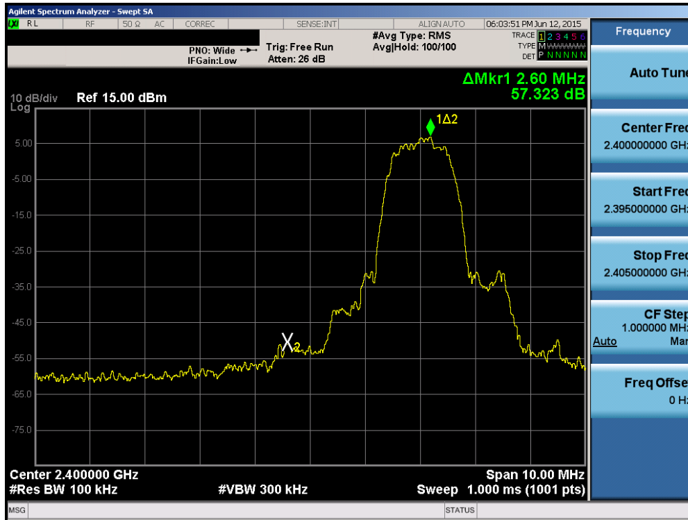
Plot 6-28. Band Edge Plot (Bluetooth with Hopping Disabled, 3 Mbps – Ch. 0)
