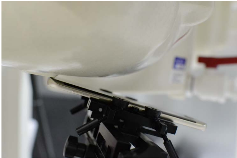
SAR Test Setup Photo 2- Right Tilt
