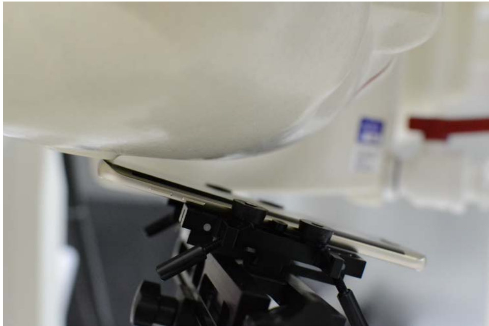
SAR Test Setup Photo 2- Right Tilt
