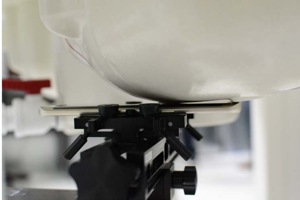
SAR Test Setup Photo 3- Left Cheek
