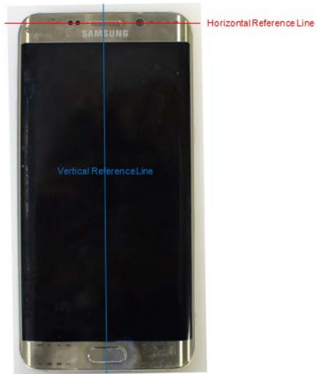
SAR Test Setup Photo 15– DUT Reference Lines
