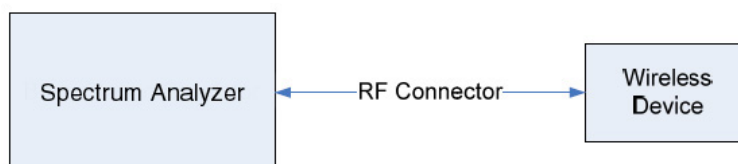
Figure 6-1. Test Instrument & Measurement Setup
