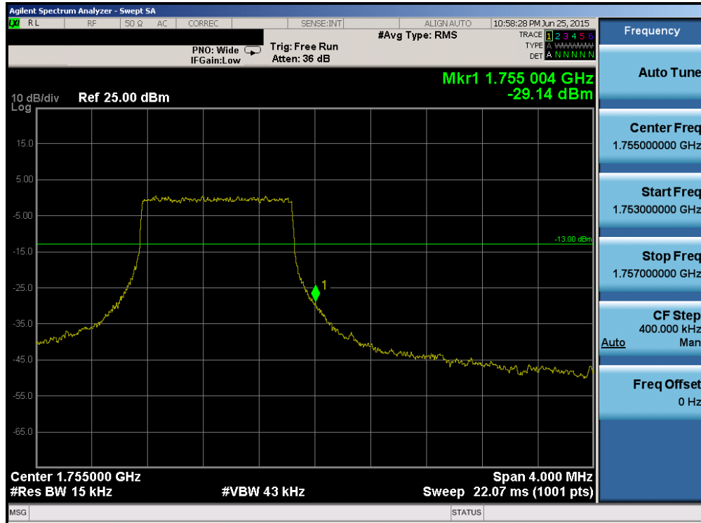
Plot 6-120. Upper Band Edge Plot (Band 4 – 1.4MHz QPSK – RB Size 6)
