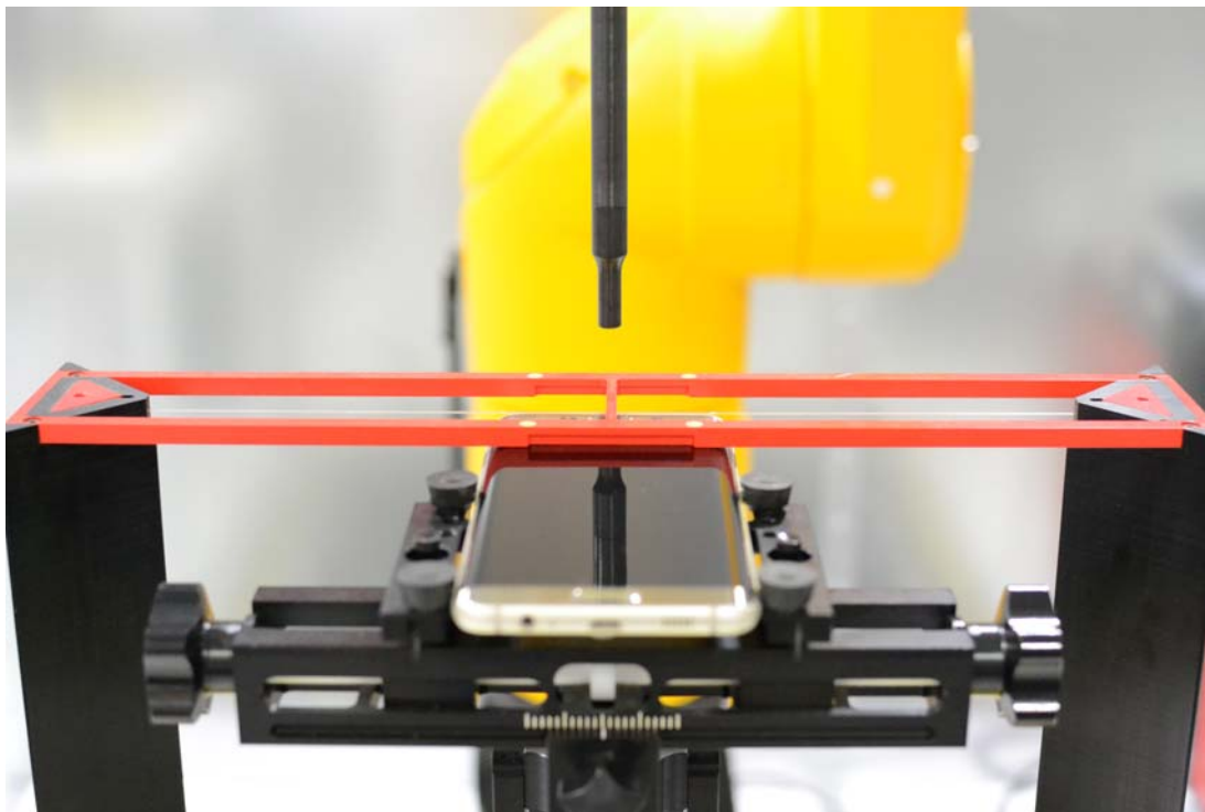
Figure 18-1 Ear Reference Point HAC Phantom Alignment
